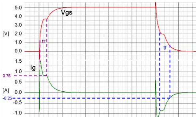
Fig. 2 Power MOSFET gate-to-source voltage, V_{gs} (top curve) and gate current (bottom curve), I_g during switching transitions
