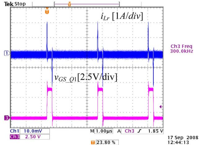
Fig. 28. Inductor current and gate-to-source voltage at 300 kHz.
