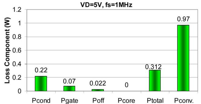
Fig. 14. Loss breakdown of the proposed CSD and total loss comparison with the conventional voltage-source driver.
