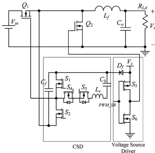
Fig. 15. Proposed discontinuous CSD diagram in the experiment.
