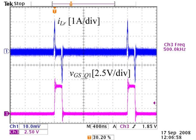
Fig. 29. Inductor current and gate-to-source voltage at 500 kHz.
