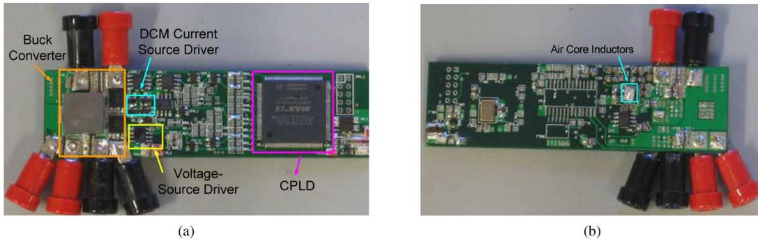
Fig. 16. Photo of the synchronous buck prototype with the hybrid gate driver. (a) Top. (b) Bottom.
