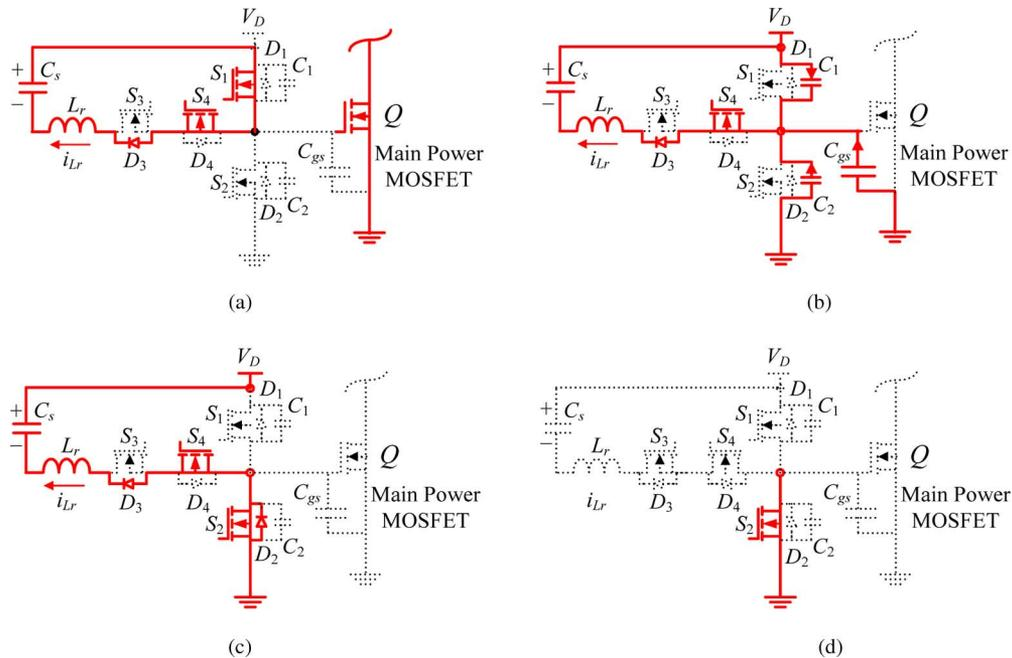
Fig. 4. Equivalent circuits: turn OFF intervals.
