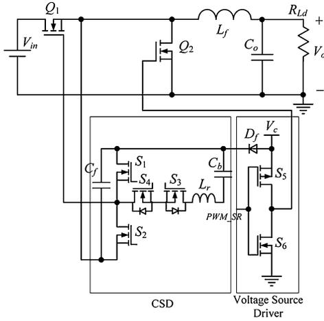
Fig. 11. Buck converter with proposed discontinuous CSD.
