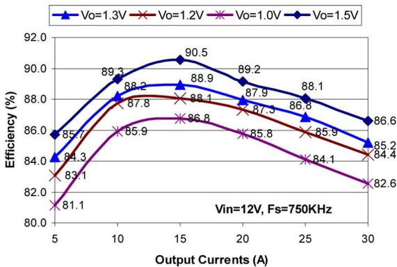
Fig. 23. Efficiency with different output voltages and currents at 750 kHz.
