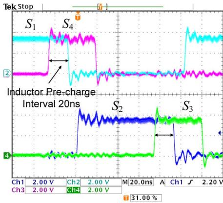
Fig. 17. Gate signals of drive MOSFETs  $S_1$ – $S_4$ .
