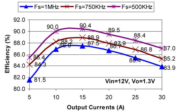
Fig. 25. Efficiency with different currents and switching frequencies at  $V_o = 1.3 V$ .
