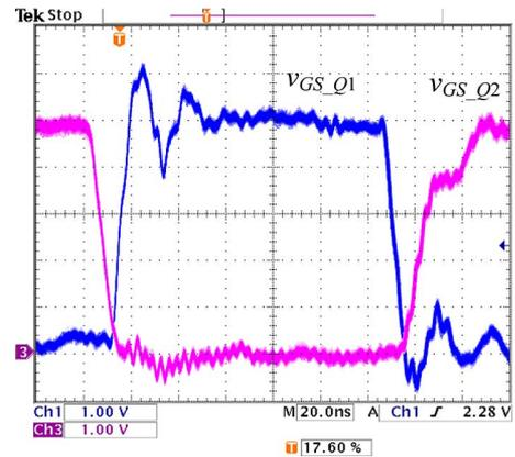
Fig. 19. Gate signals  $v_{GS\_Q1}$  (control MOSFET) and  $v_{GS\_Q2}$  (SR).
