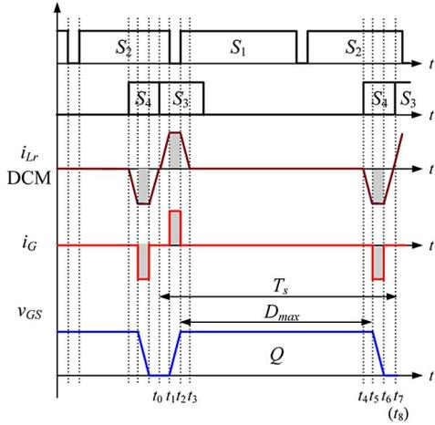
Fig. 7. Key waveforms with maximum duty cycle.
