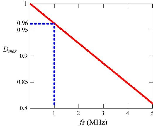
Fig. 8. Maximum duty cycle versus the switching frequency.
