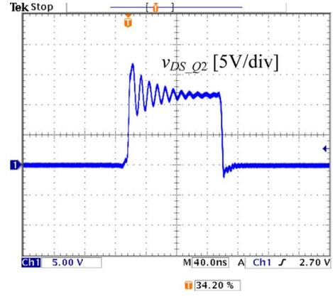
Fig. 20. Drain-to-source voltage  $v_{DS\_Q2}$  (SR) at load current of 25 A.
