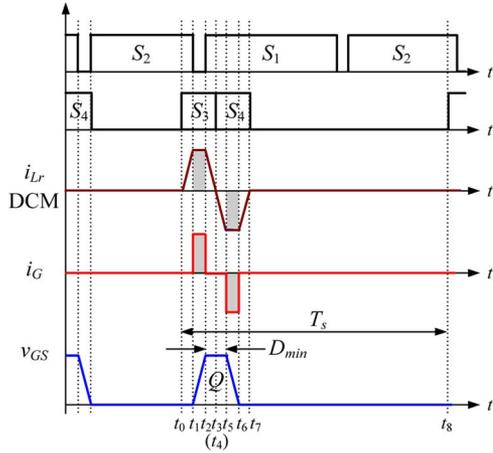
Fig. 5. Key waveforms with minimum duty cycle.
