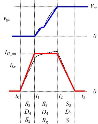
Fig. 12. Detailed inductor current and power MOSFET gate voltage waveforms during the turn ON interval.
