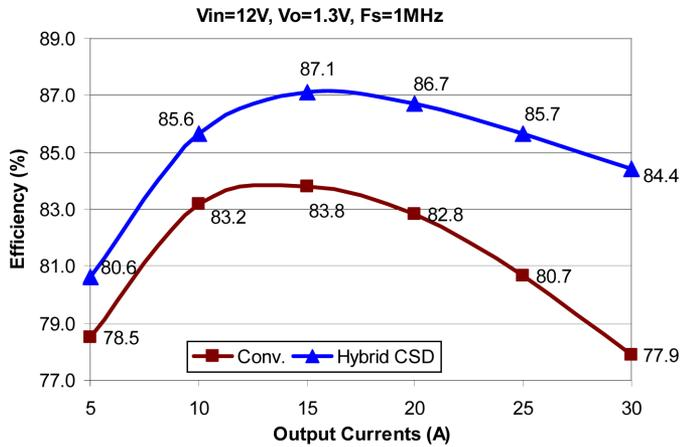
Fig. 21. Efficiency comparison. (Top) Hybrid CSD. (Bottom) Conventional voltage driver (conv.).
