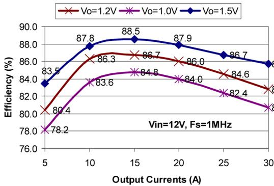
Fig. 22. Efficiency with different output voltages and currents at 1 MHz.
