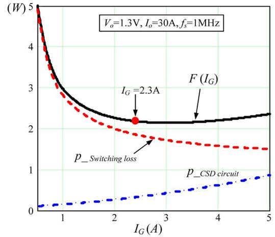
Fig. 13. Objective function  $F(I_G)$  as function of current  $I_G$ .
