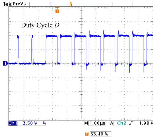
Fig. 30. Gate signals  $v_{GS\_Q1}$  (control MOSFET) from  $D = 0.1$  to  $0.8$ .
