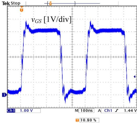
Fig. 27. Gate signals  $v_{GS}$  at 2 MHz.
