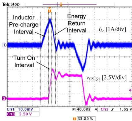
Fig. 18. Inductor current and the gate-to-source voltage at 1 MHz.
