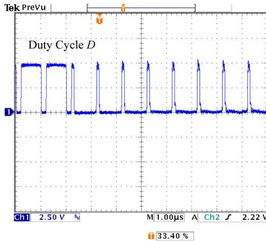
Fig. 31. Gate signals  $v_{GS\_Q1}$  (control MOSFET) from  $D = 0.8$  to  $0.1$ .
