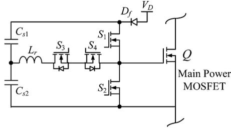
Fig. 10. Proposed high-side CSD using series capacitors.
