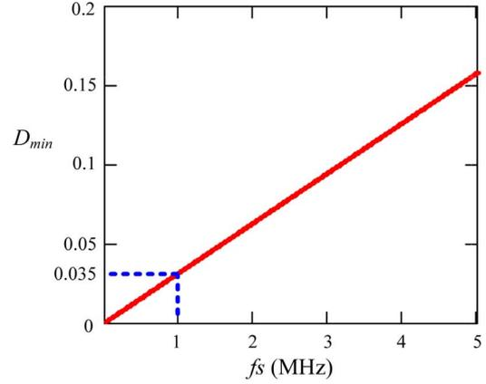
Fig. 6. Minimum duty cycle versus the switching frequency.
