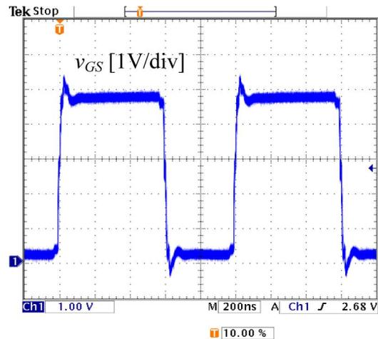
Fig. 26. Gate signals  $v_{GS}$  at 1 MHz.
