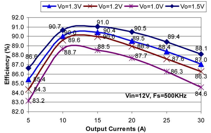
Fig. 24. Efficiency with different output voltages and currents at 500 kHz.
