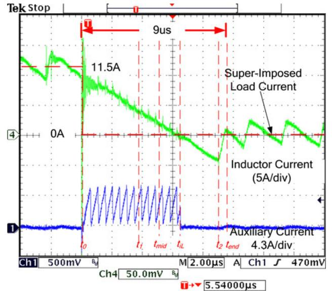
Fig. 20. Digital charge balance controller's response to a 11.5 A  $\rightarrow$  0 A load step without load-line regulation (inductor current and auxiliary current).
