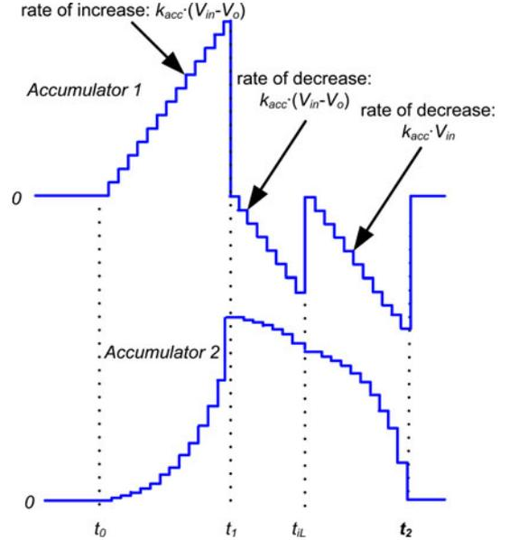
Fig. 7. Digital double accumulator to determine  $t_2$  without load-line regulation.
