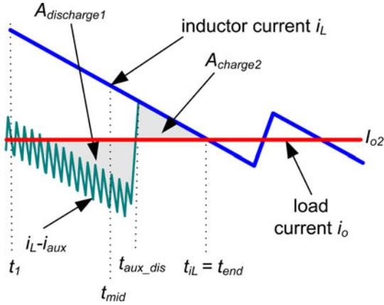
Fig. 10. Capacitor charge areas for Case #2.
