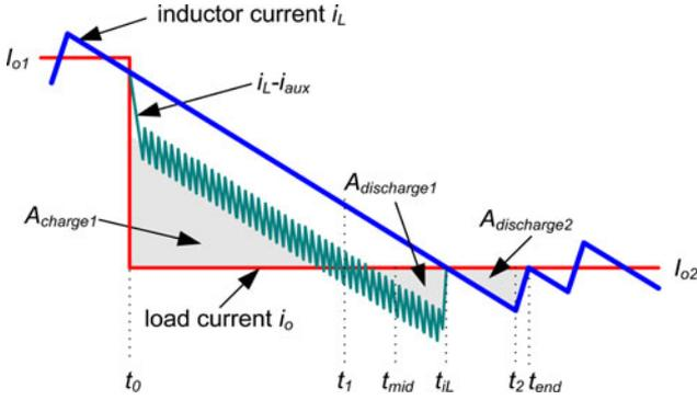
Fig. 8. Capacitor charge regions for load-line regulation (Case #1).
