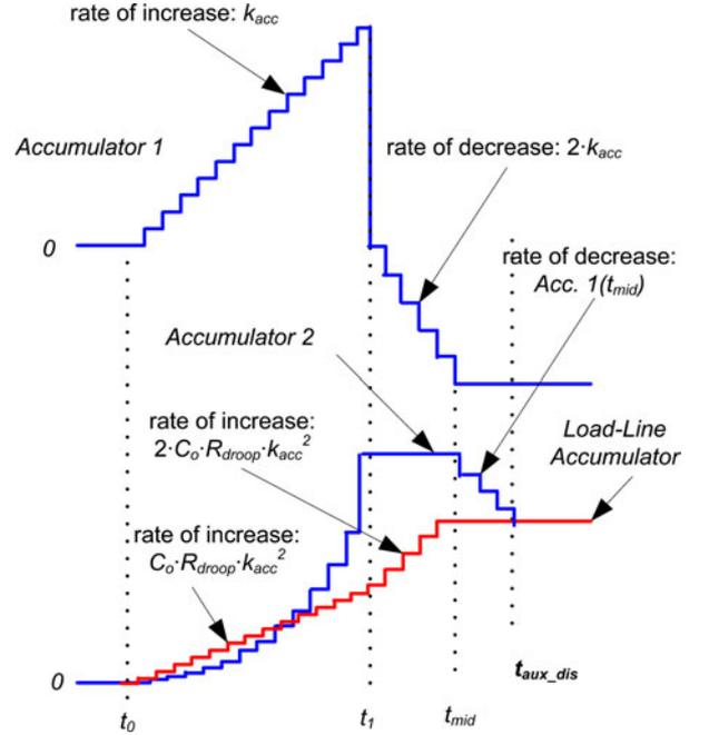
Fig. 11. Digital double accumulator to determine  $t_{aux\_dis}$  with load-line regulation (Case #2).
