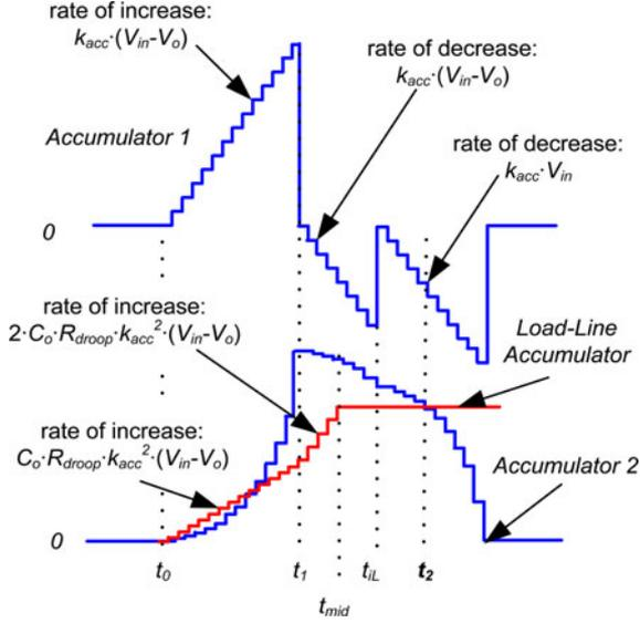
Fig. 9. Digital double accumulator to determine  $t_2$  with load-line regulation (Case #1).
