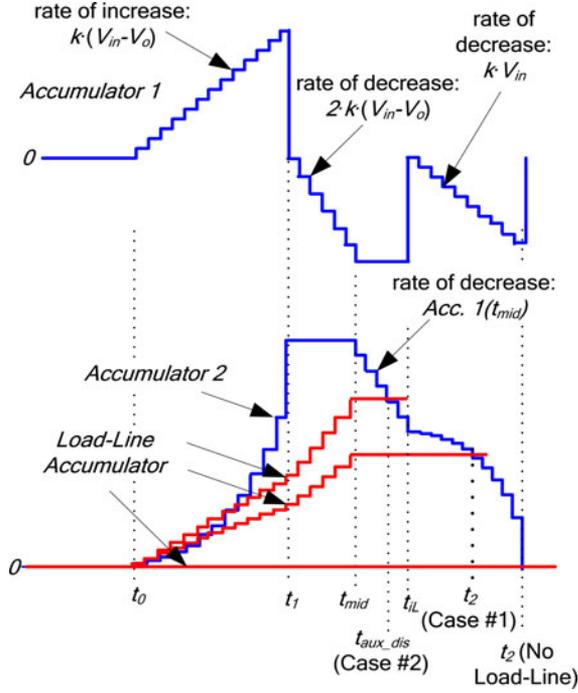
Fig. 12. Digital double accumulator operation for all possible cases.
