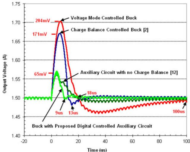
Fig. 16. Simulated response to a 10 A  $\rightarrow$  0 A load current step change without load-line regulation ( $I_{aux\_avg} = 3.8$  A).
