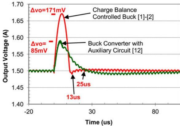
Fig. 3. Charge balance control response [1], [2] versus auxiliary circuit response [12].
