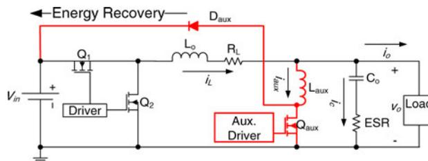
Fig. 2. Implementation of high-frequency auxiliary circuit [12].
