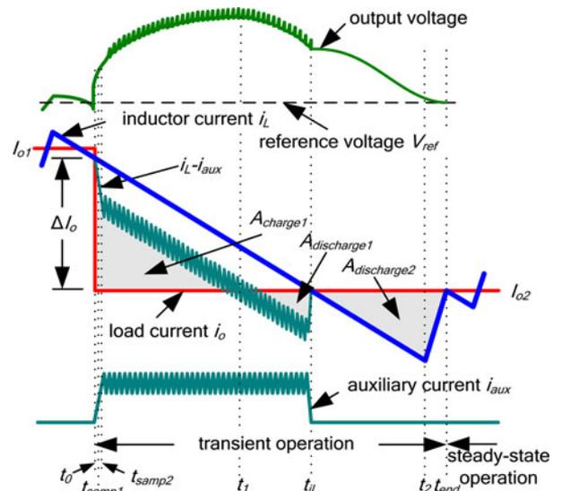
Fig. 4. Proposed controller reaction to an unloading transient (w/o load-line regulation).
