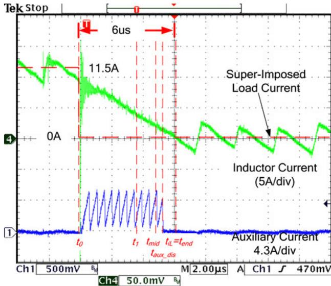
Fig. 25. Digital charge balance controller's response to an 11.5 A  $\rightarrow$  0 A load step with load-line regulation (inductor current and auxiliary current).
