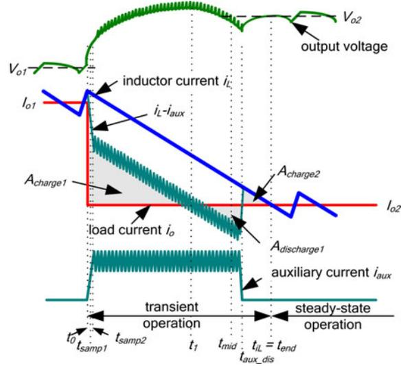
Fig. 6. Controller reaction to an unloading transient with load-line regulation (Case #2).
