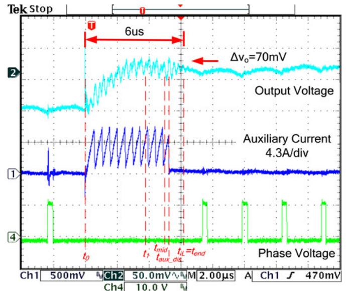
Fig. 24. Digital charge balance controller's response to an 11.5 A  $\rightarrow$  0 A load step with load-line regulation.
