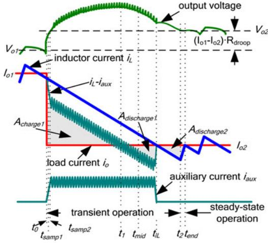
Fig. 5. Controller reaction to an unloading transient with load-line regulation (Case #1).
