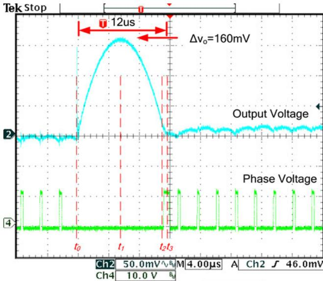
Fig. 19. Digital charge balance controller's response (without auxiliary circuit) to a 11.5 A  $\rightarrow$  0 A load step without load-line regulation.
