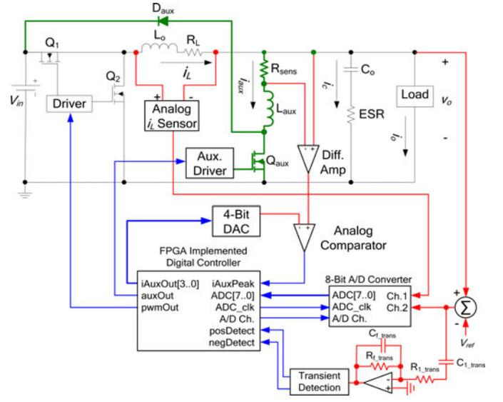
Fig. 13. System-level block diagram of digitally implemented charge balance controller with auxiliary circuit.
