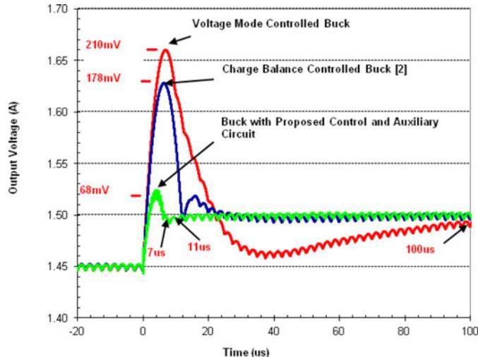
Fig. 17. Simulated response to a 10 A  $\rightarrow$  0 A load current step change with load-line regulation ( $I_{aux\_avg} = 3.8$  A).
