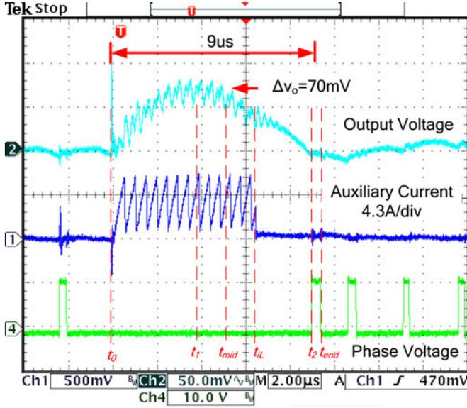
Fig. 18. Digital charge balance controller's response to a 11.5 A  $\rightarrow$  0 A load step without load-line regulation.
