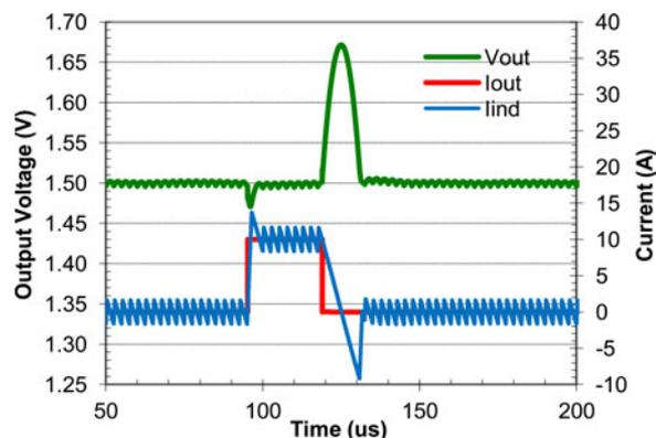
Fig. 1. Asymmetrical transient response to positive/negative load current step change (charge balance controller response).
