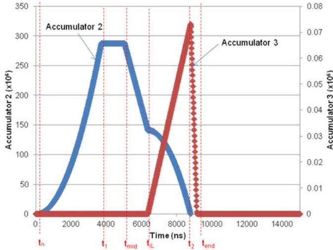
Fig. 21. Digital control signals of charge balance controller during 11.5 A  $\rightarrow$  0 A load current transient without load-line regulation.
