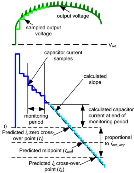
Fig. 15. Prediction of  $t_1$ ,  $t_{mid}$ , and  $t_{iL}$  by capacitor current zero-crossover predictor.
