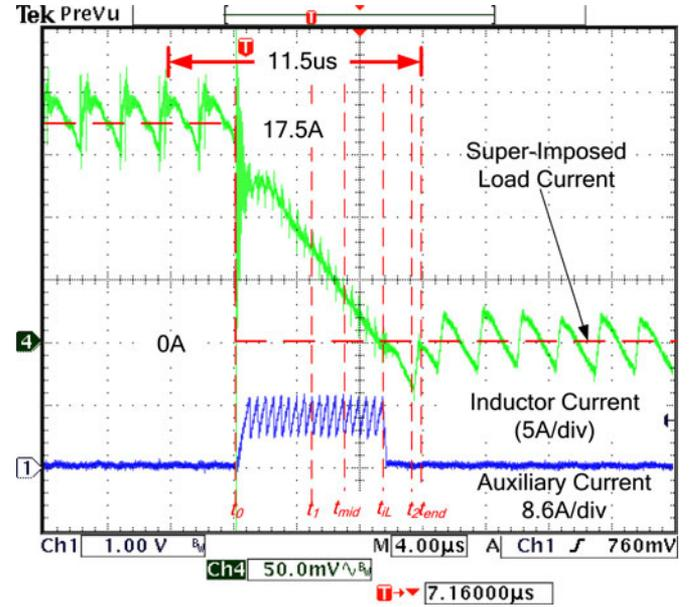
Fig. 23. Digital charge balance controller's response to a 17.5 A  $\rightarrow$  0 A load step without load-line regulation (inductor current and auxiliary current).
