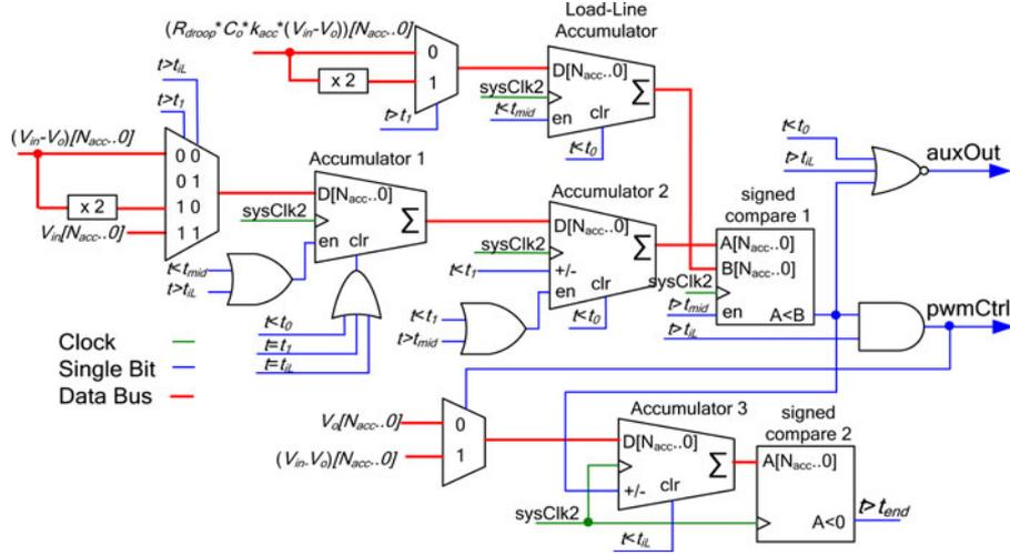
Fig. 14. Logic diagram of double accumulator structure.
