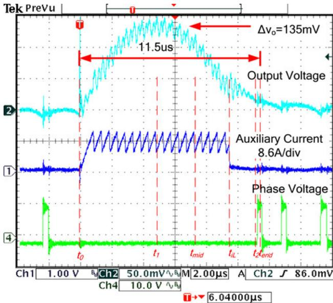
Fig. 22. Digital charge balance controller's response to a 17.5 A  $\rightarrow$  0 A load step without load-line regulation (output voltage, auxiliary current, and phase voltage).
