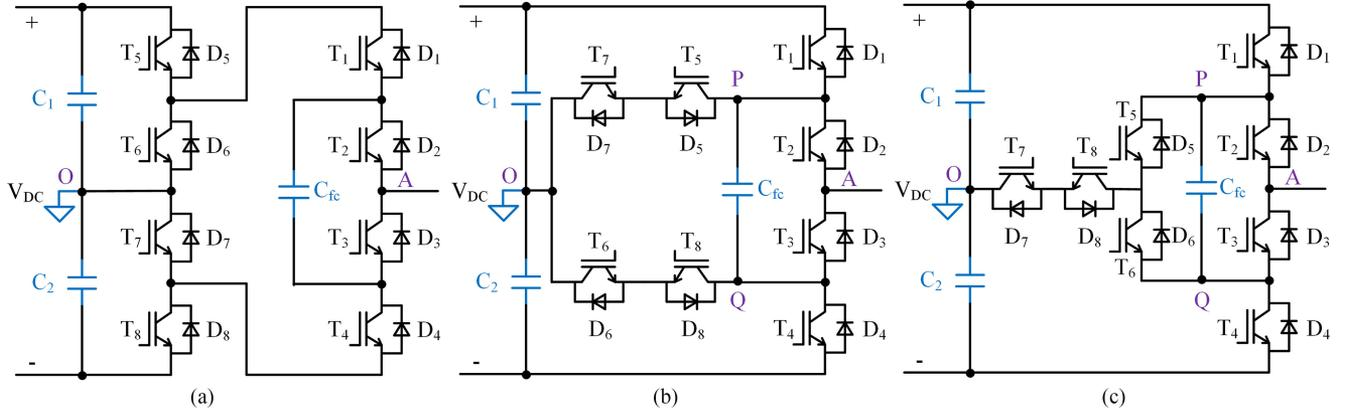
Fig. 2. 5L-ANPC inverter topologies. (a) Type I. (b) Type II. (c) Type III.
