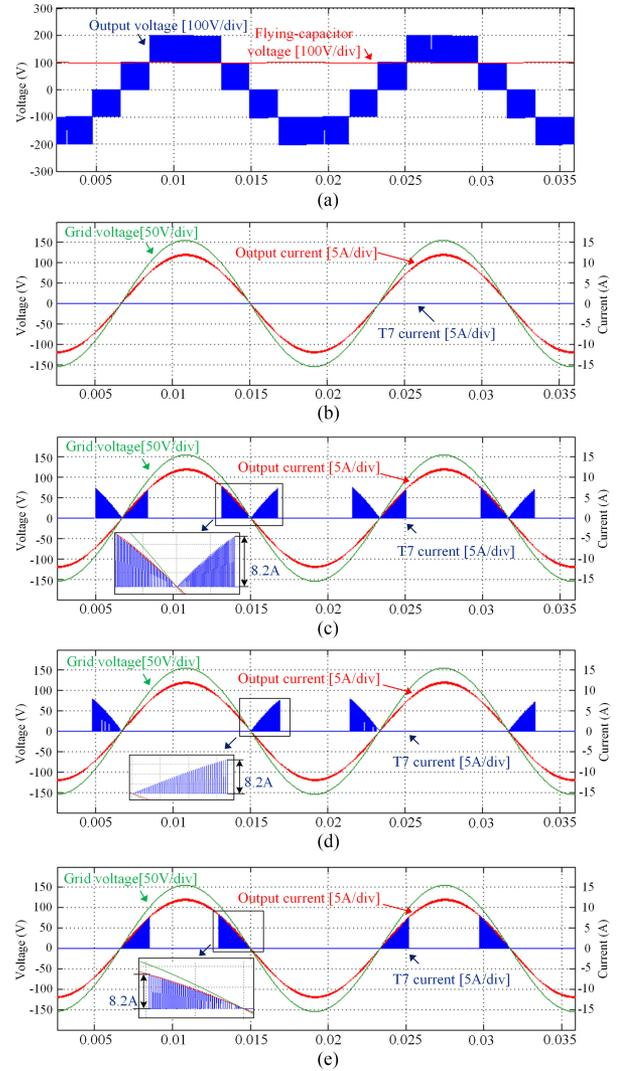
Fig. 14. Simulation results under unity power factor condition. (a) Output voltage and FC voltage. (b)  $T_7$  current in case 1. (c)  $T_7$  current in case 2. (d)  $T_7$  current in case 3. (e)  $T_7$  current in case 4.
