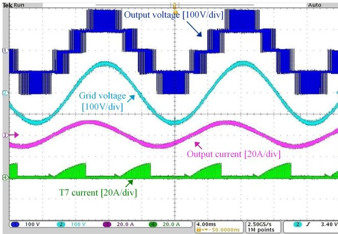
Fig. 22. Waveform of  $T_7$  current in modulation case 2 (PF = 0.9, capacitive).
