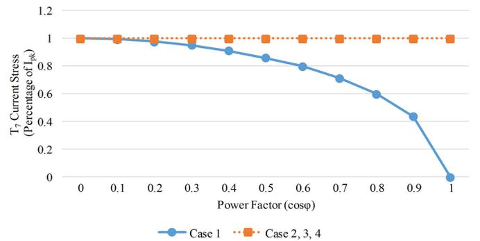
Fig. 9. Comparison of  $T_7$  current stress in four cases ( $M = 0.45$ ).
