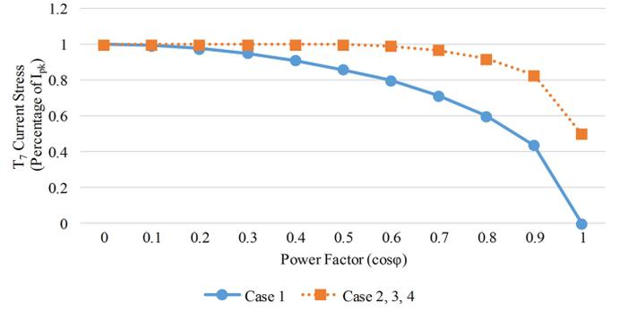
Fig. 7. Comparison of  $T_7$  current stress in four cases ( $M = 1$ ).
