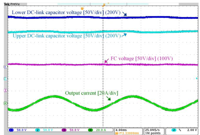
Fig. 20. Experimental results under reactive power condition ( $\text{PF} = 0.9$ , capacitive): waveforms of lower dc-link capacitor voltage, upper dc-link capacitor voltage, FC voltage, and output current.
