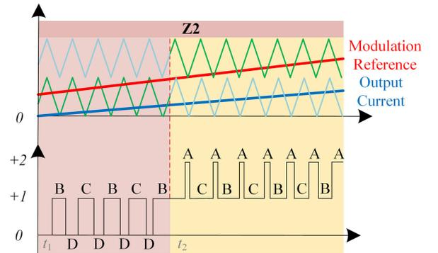
Fig. 12. PWM Modulation in active power zone Z2.
