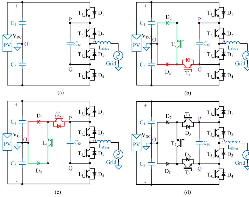
Fig. 3. Derivation of the proposed 7S-5L-ANPC inverter topology. (a) Circuit 1. (b) Circuit 2. (c) Circuit 3. (d) Proposed topology.
