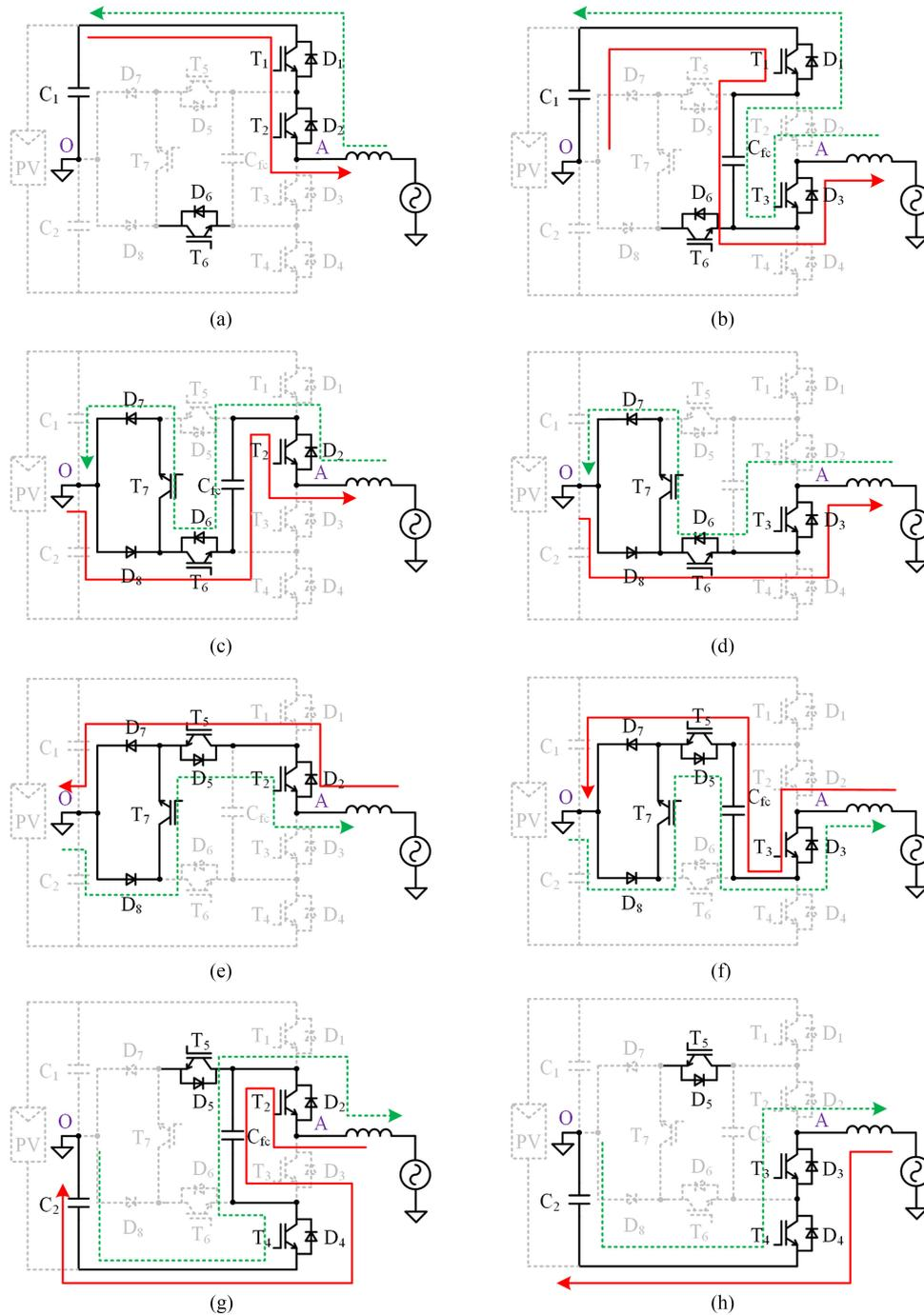
Fig. 4. Eight switching states for 7S-5L-ANPC inverter. (a) State A: +2. (b) State B: +1. (c) State C: +1. (d) State D: 0. (e) State E: 0. (f) State F: -1. (g) State G: -1. (h) State H: -2.
