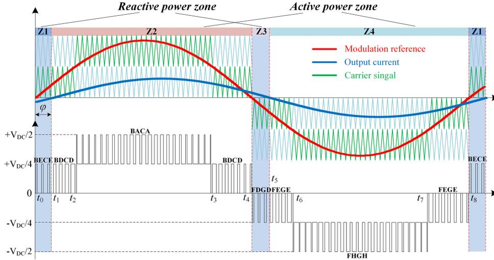
Fig. 10. PWM modulation for 7S-5L-ANPC inverter.
