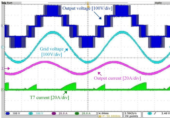
Fig. 23. Waveform of  $T_7$  current in modulation case 3 (PF = 0.9, capacitive).
