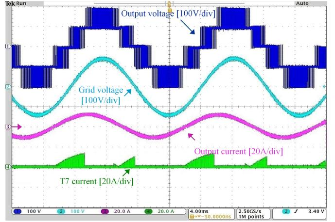
Fig. 24. Waveform of  $T_7$  current in modulation case 4 (PF = 0.9, capacitive).
