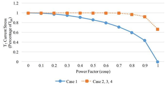
Fig. 8. Comparison of  $T_7$  current stress in four cases ( $M = 0.78$ ).
