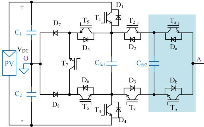
Fig. 5. Extension of voltage levels based on 7S-5L-ANPC topology (seven-level topology).
