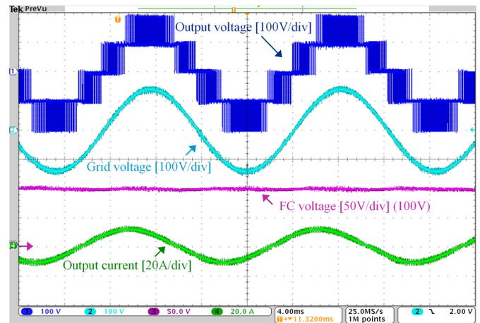
Fig. 19. Experimental results under reactive power operation ( $\text{PF} = 0.9$ , capacitive): waveforms of inverter bridge voltage, grid voltage, FC voltage, and output current.
