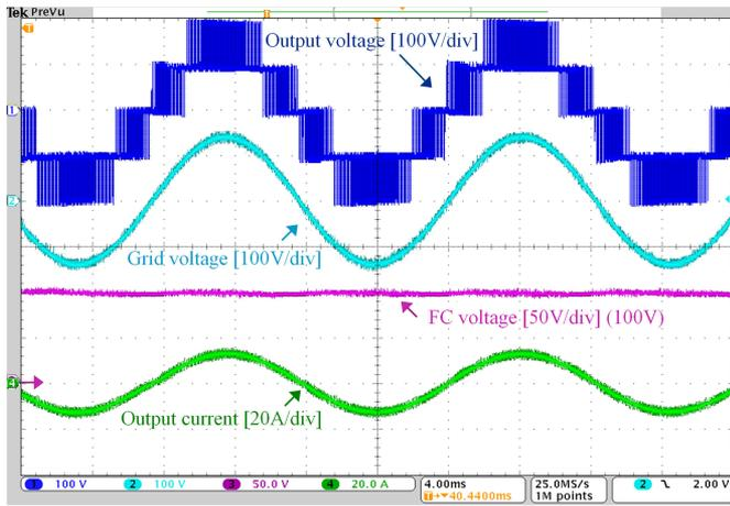
Fig. 17. Experimental results under unity power factor condition: waveforms of inverter output voltage, grid voltage, FC voltage, and output current.
