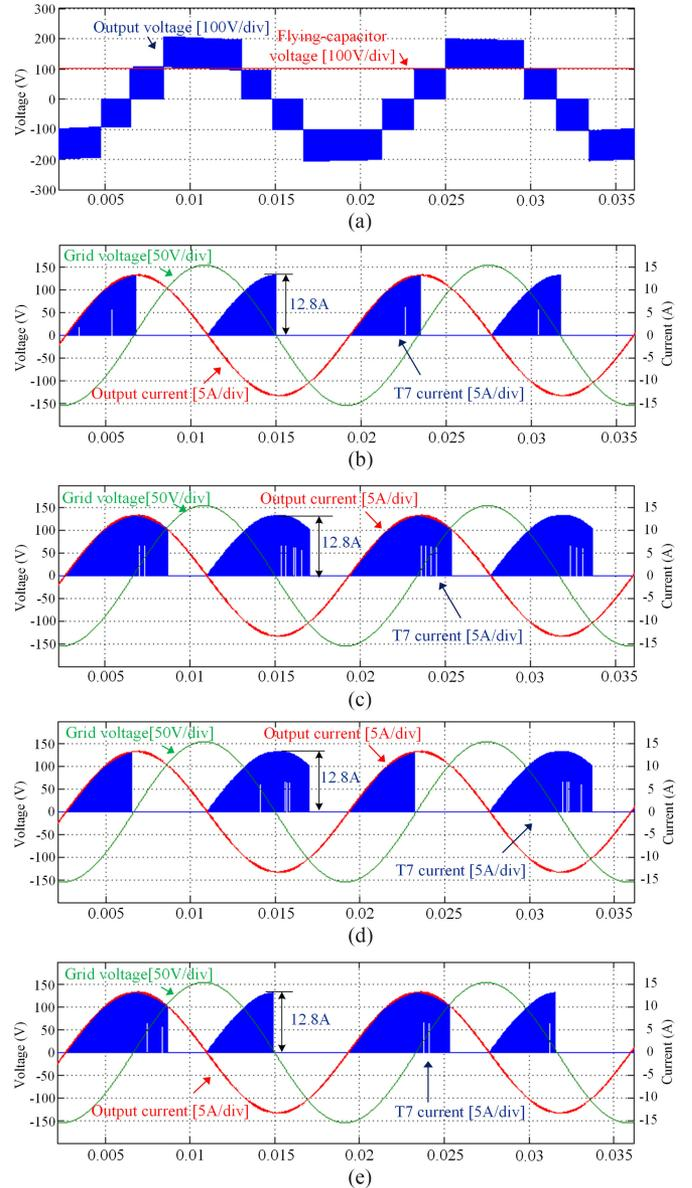
Fig. 16. Simulation results under reactive power condition (PF = 0). (a) Output voltage and FC voltage. (b)  $T_7$  current in case 1. (c)  $T_7$  current in case 2. (d)  $T_7$  current in case 3. (e)  $T_7$  current in case 4.
