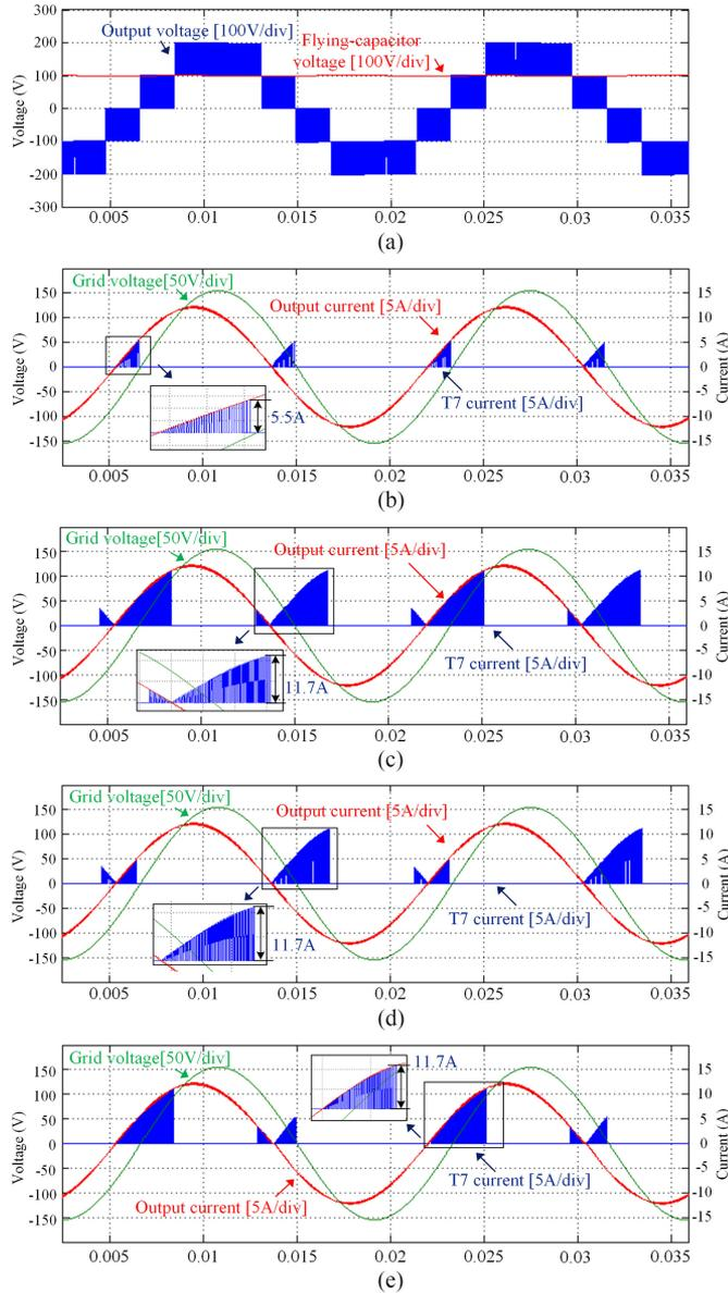
Fig. 15. Simulation results under reactive power condition (PF = 0.9, capacitive). (a) Output voltage and FC voltage. (b)  $T_7$  current in case 1. (c)  $T_7$  current in case 2. (d)  $T_7$  current in case 3. (e)  $T_7$  current in case 4.
