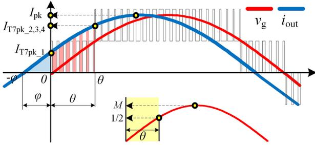
Fig. 6. Waveforms of output current and grid voltage under reactive power condition.
