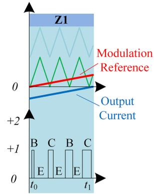
Fig. 11. Modulation in reactive power zone Z1.
