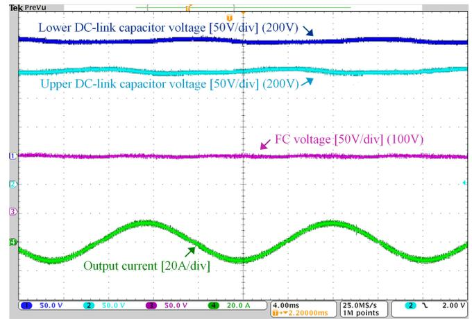
Fig. 18. Experimental results under unity power factor condition: waveforms of lower dc-link capacitor voltage, upper dc-link capacitor voltage, FC voltage, and output current.
