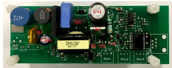
Fig. 14 7.5W MRC LED Driver experimental prototype
