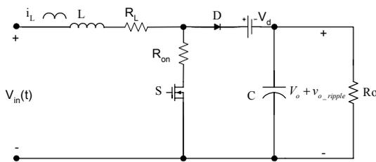
Figure 5. Accurate model of Boost converter
