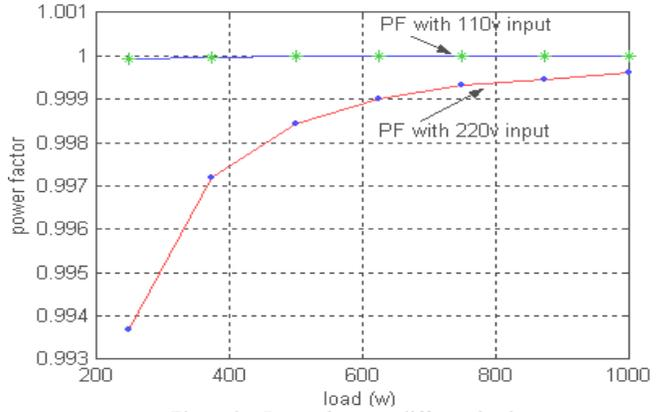
Figure 9. Power factor at different load
