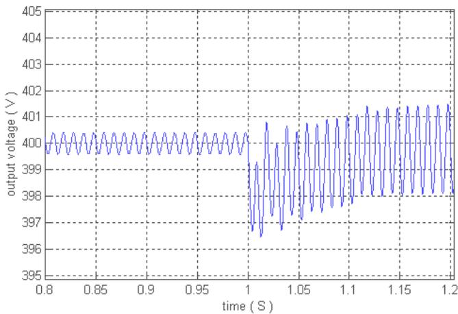
Figure 12. Voltage waveform during step load changed from 250w to 1000w
