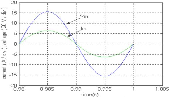
(a) Input current and voltage waveform
