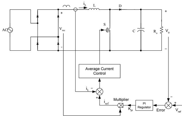
Figure 1. Average current control of the Boost PFC
