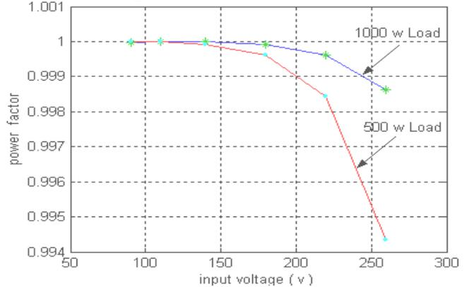
Figure 10. Power factor with different input voltage
