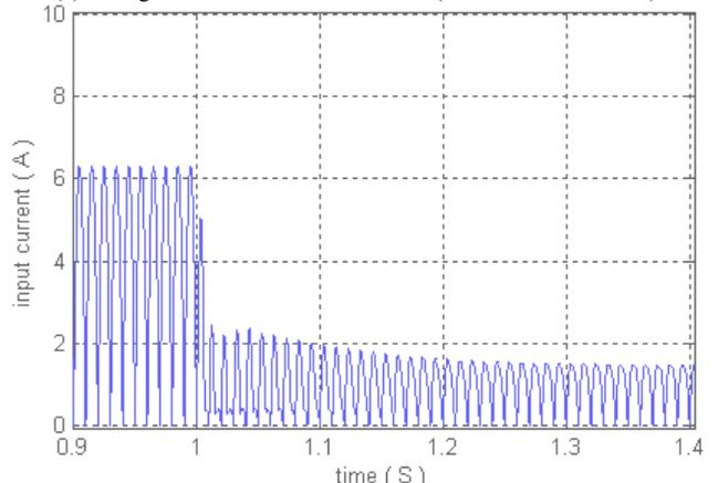
(b) Current waveform in transient state (Load: 1000w to 250w)
