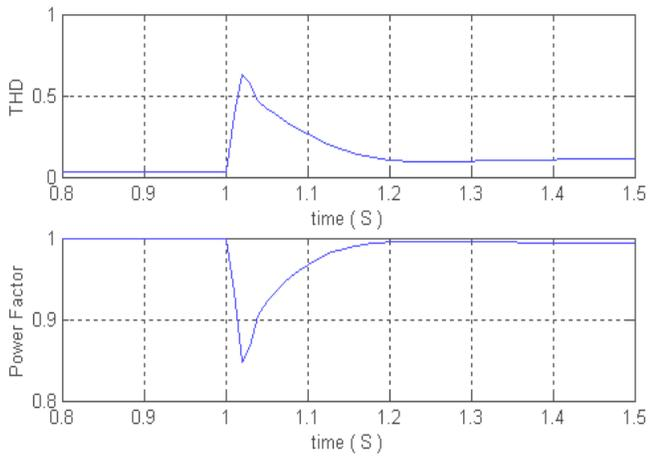
(c) THD and power factor in transient state (Load: 1000w to 250w)
