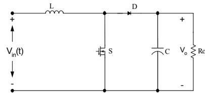
Figure 2. Boost converter topology
