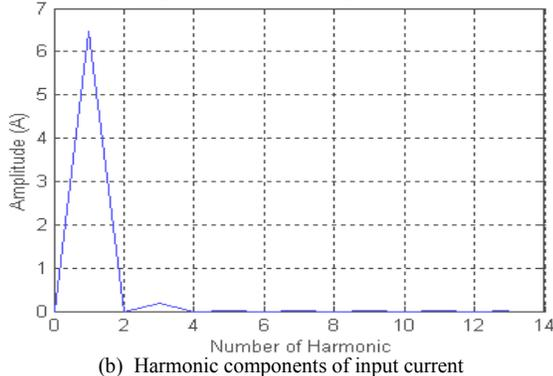
(b) Harmonic components of input current
