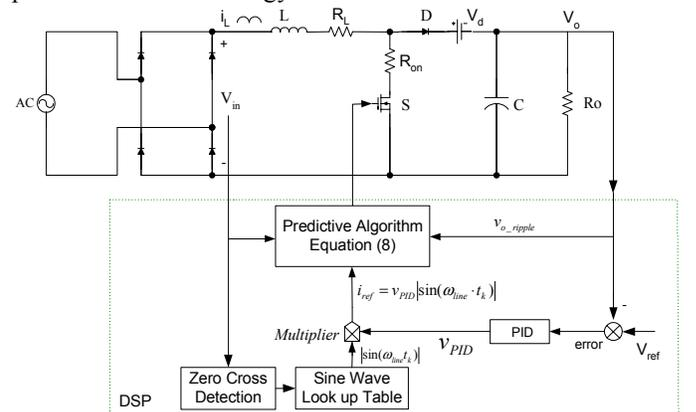
Figure 6. Digital predictive control for Boost PFC preregulator
