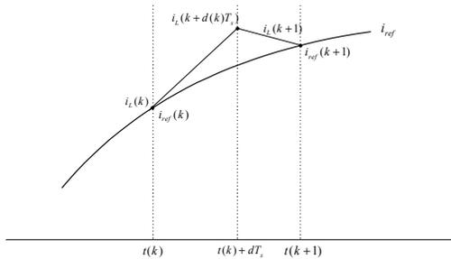
Figure 4. Input current waveform and reference current in one  $T_s$
