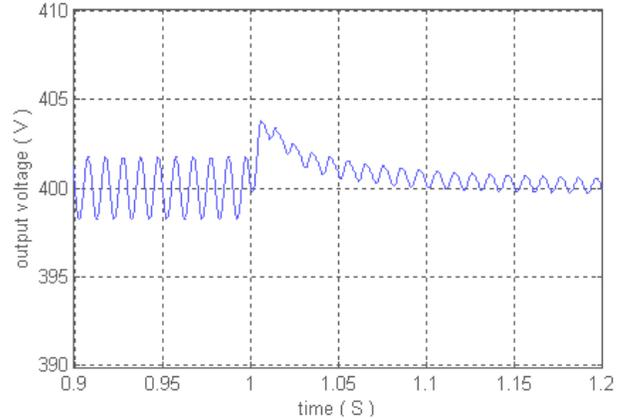
(a) Voltage waveform in transient state (Load: 1000w to 250w)
