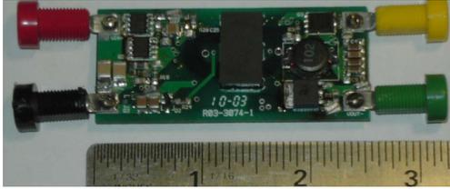
Figure 8 48V/5V, 30W, 400kHz AHB prototype
