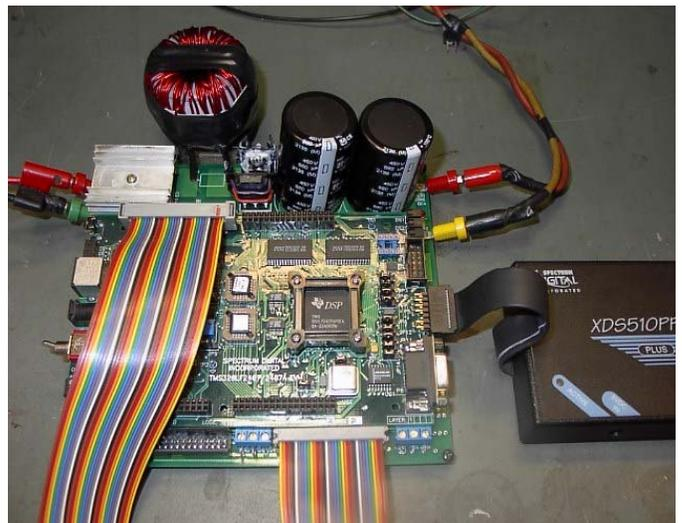
Fig. 10 Boost PFC circuit controlled by DSP evaluation board
