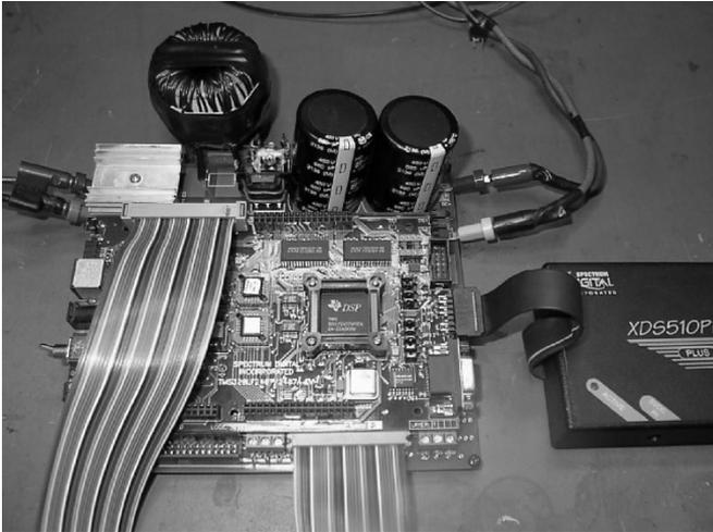
Fig. 14. Boost PFC circuit controlled by DSP evaluation board.
