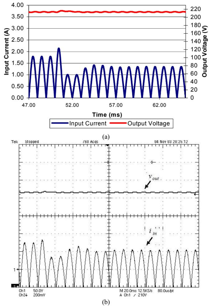
Fig. 11. Results for  $I_{in}$  and  $V_{out}$  when  $V_{in}$  is stepped from 95V to 110V RMS: (a) Model simulation (b) Experimental results
