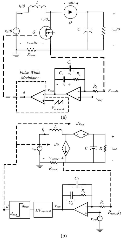
Fig. 3. (a) DC-to-DC Boost converter with average current control and PWM circuit (b) The proposed model: averaged DC-to-DC Boost converter model with average current control and PWM circuit model
