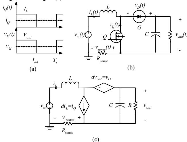
Fig. 1. (a) Switching and averaged waveforms of the Boost converter: the dashed line represents the averaged value of the waveform (b) Boost converter with  $R_{sense}$  (c) Averaged model for a Boost converter with  $R_{sense}$ .
