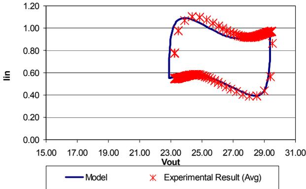
Fig. 7. Phase plane plot when the control signal  $v_{iref}$  is stepped between 0.5A and 1A – solid line: model simulation, dashed line: experimental results
