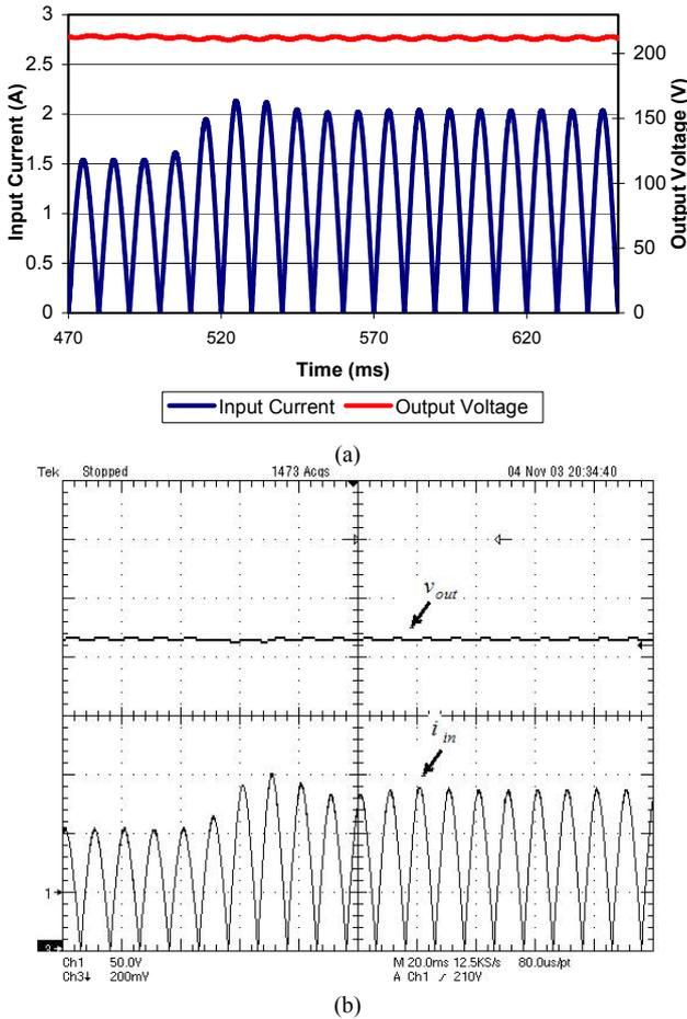
Fig. 10. Results for  $I_{in}$  and  $V_{out}$  when  $R_{Load}$  is stepped from 400Ω to 300Ω: (a) Model simulation (b) Experimental results
