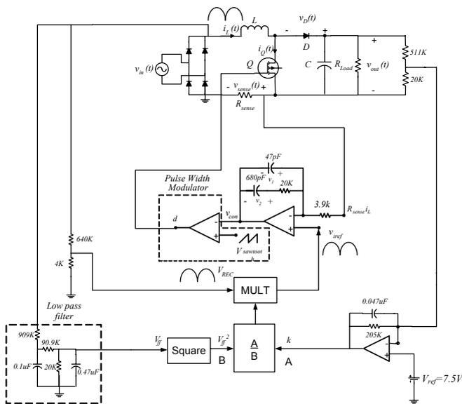
Fig. 5. Single-phase Boost PFC converter with average current control.
