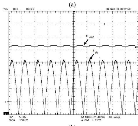
Fig. 9. The steady-state input current and output voltage waveforms: (a) Model simulation (b) Experimental results
