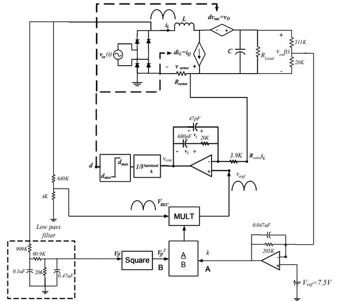
Fig. 6. The proposed single-phase Boost PFC model.
