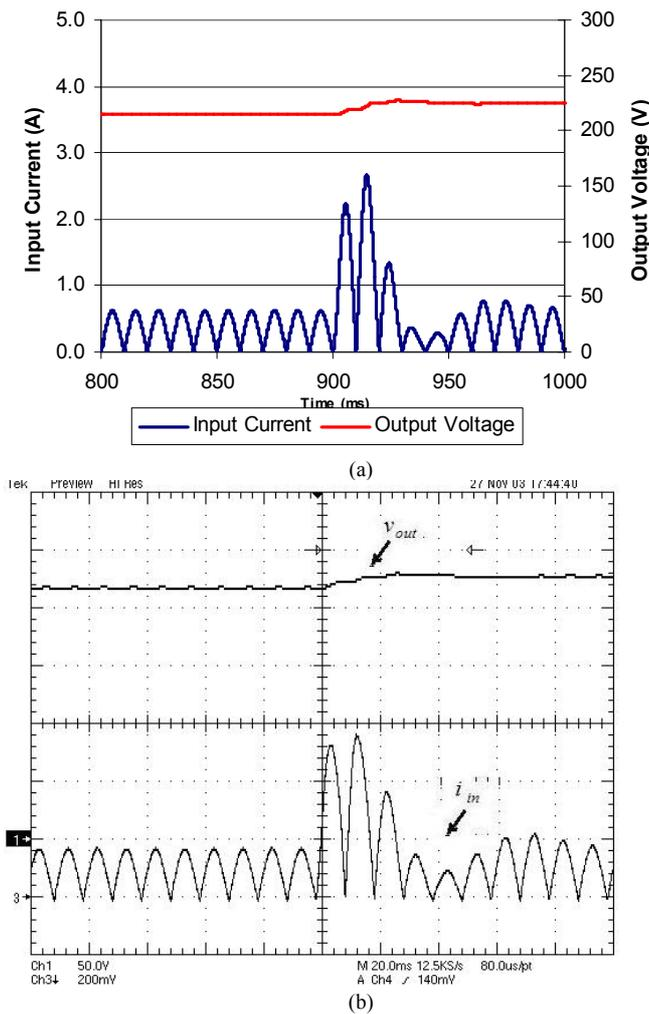
Fig. 12. Results for  $I_{in}$  and  $V_{out}$  when  $V_{out}$  is stepped from 215V to 225V: (a) Model simulation (b) Experimental results
