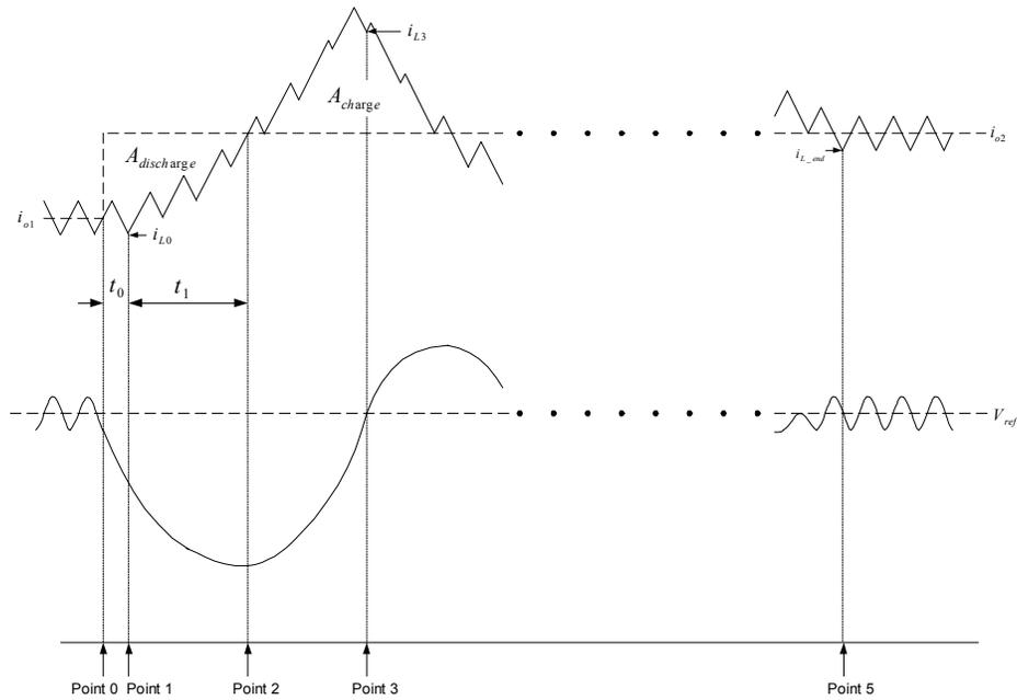
Fig. 2 Transient response of a voltage mode controlled buck converter under positive load current step change (top: inductor current, bottom: capacitor voltage)
