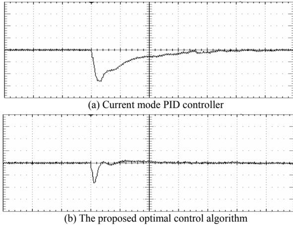
Fig. 5 Experimental result of output voltage response to load current change from 0A to 5A (X axis: 40us/div; Y axis: 50mv/div)
