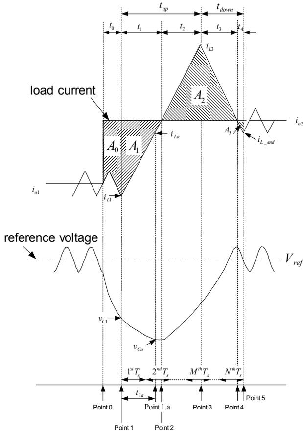
Fig. 3 Optimal inductor current transient for load current positive change when  $t_{opt} = NT_s$  (top: inductor current, bottom: capacitor voltage)
