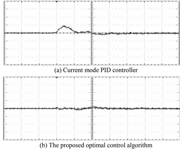
Fig. 7 Experimental result of output voltage response to input voltage change from 5V to 7.5V (X axis: 40us/div; Y axis: 50mv/div)
