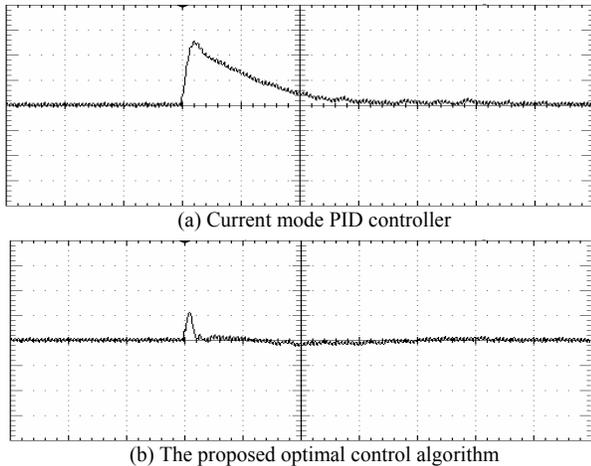
Fig. 6 Experimental result of output voltage response to load current change from 5A to 0A (X axis: 40us/div; Y axis: 50mv/div)
