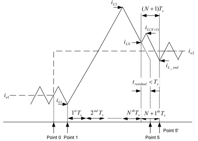
Fig. 4 Optimal inductor current transient for load current positive change when  $T_{opt} = NT_s + T_{residual}$
