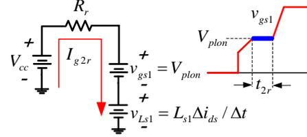
Fig. 10. Driver equivalent circuit during  $t_{2r}$
