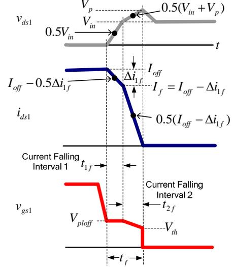
Fig. 12. Synchronous buck HS MOSFET waveforms at turn off with piecewise linear approximations
