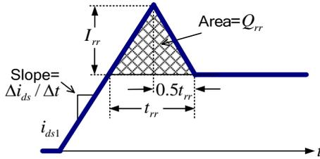
Fig. 11. Synchronous buck HS MOSFET current waveform approximation during reverse recovery at turn on
