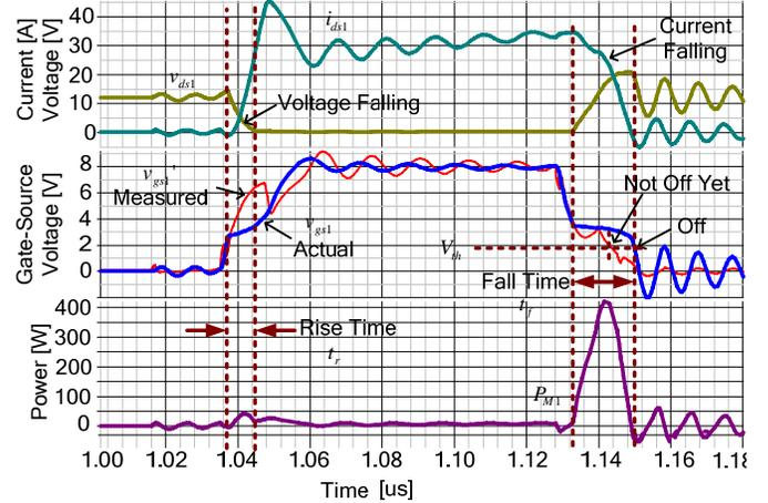
Fig. 2. Synchronous buck voltage regulator HS MOSFET waveforms (top: actual drain-source voltage,  $v_{ds1}$  and drain current,  $i_{ds1}$ ; middle: measured gate-source voltage,  $v_{gs1}'$  and actual gate-source voltage (bold),  $v_{gs1}$ ; bottom: HS MOSFET power,  $v_{ds1}i_{ds1}$ )
