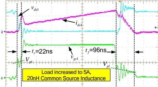
Fig. 4. Switching waveforms at 5A load and 20nH common source inductance (80ns/div;  $v_{ds1}$ : 10V/div;  $i_{ds1}$ : 5A/div;  $v_{gs1}$ : 5V/div)
