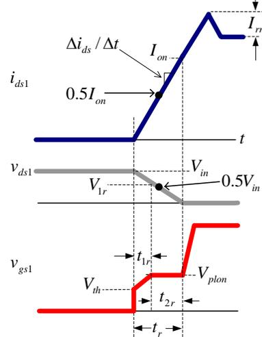
Fig. 7. Synchronous buck HS MOSFET waveforms at turn on with piecewise linear approximations
