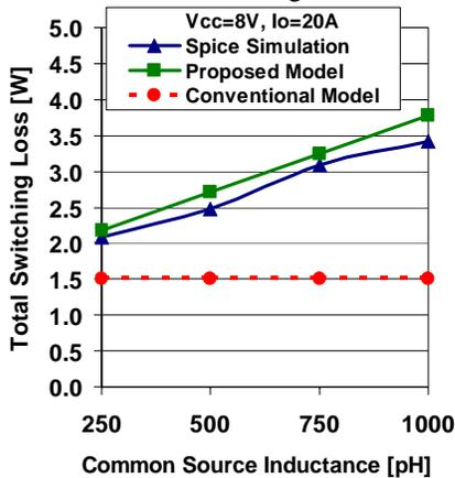
Fig. 16. Total switching loss at 1MHz, 12V input vs. common source circuit inductance ( $V_{cc}=8V, I_o=20A$ )
