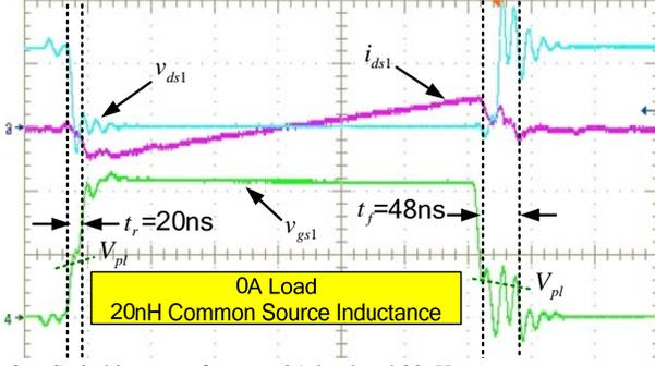
Fig. 3. Switching waveforms at 0A load and 20nH common source inductance (80ns/div;  $v_{ds1}$ : 10V/div;  $i_{ds1}$ : 5A/div;  $v_{gs1}$ : 5V/div)
