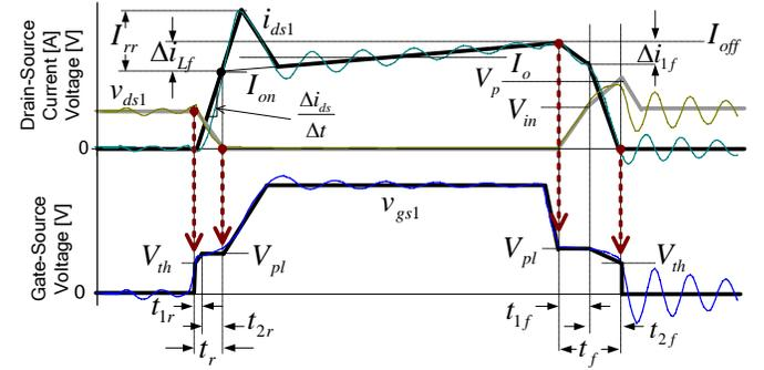
Fig. 6. Synchronous buck HS MOSFET waveforms with piecewise linear approximations of these waveforms in bold
