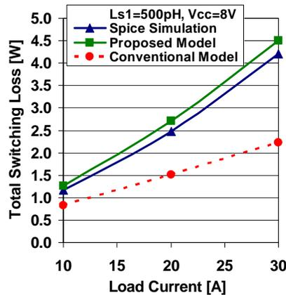
Fig. 17. Total switching loss at 1MHz, 12V input vs. load current ( $V_{cc}=8V, L_{s1}=500pH$ )
