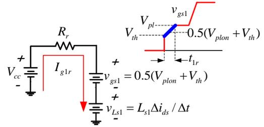
Fig. 9. Driver equivalent circuit during  $t_{2r}$
