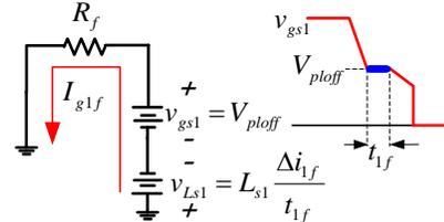
Fig. 13. Driver equivalent circuit during  $t_{1f}$
