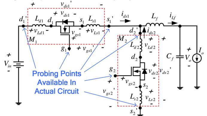
Fig. 1. Synchronous buck voltage regulator with parasitic inductances
