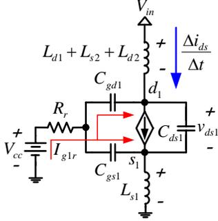
Fig. 8. Synchronous buck HS MOSFET equivalent circuit during  $t_{1r}$
