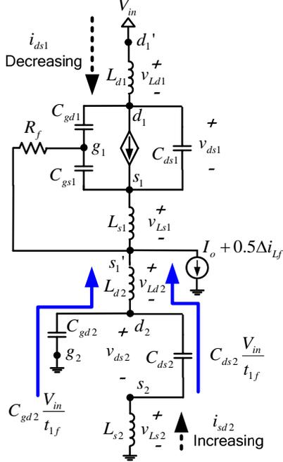
Fig. 14. Synchronous buck equivalent circuit during turn off during  $t_{1f}$
