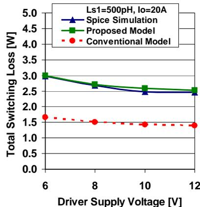
Fig. 18. Total switching loss at 1MHz, 12V input vs. driver supply voltage ( $L_{s1}=500pH, I_o=20A$ )
