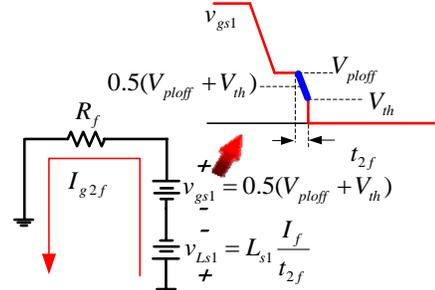
Fig. 15. Driver equivalent circuit during  $t_{2f}$
