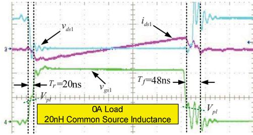
Fig. 3. Switching waveforms at 0A load and 20nH common source inductance (80ns/div;  $v_{ds1}$ : 10V/div;  $i_{ds1}$ : 5A/div;  $v_{gs1}$ : 5V/div)
