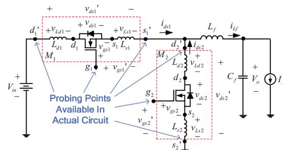
Fig. 1. Synchronous buck voltage regulator with parasitic inductances
