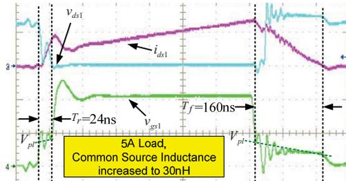
Fig. 5. Switching waveforms at 5A load with 30nH common source inductance (80ns/div;  $v_{ds1}$ : 10V/div;  $i_{ds1}$ : 5A/div;  $v_{gs1}$ : 5V/div)
