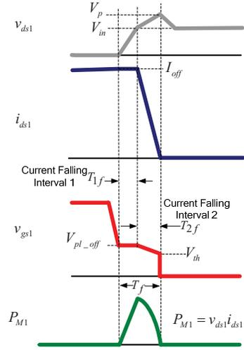
Fig. 11. Synchronous buck HS MOSFET waveforms at turn off with piecewise linear approximations
