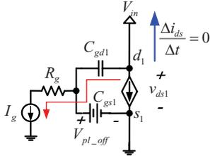
Fig. 12. Synchronous buck HS MOSFET equivalent circuit during  $T_{1f}$
