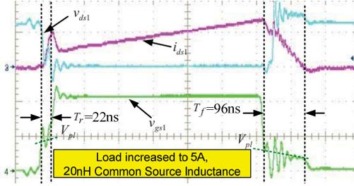
Fig. 4. Switching waveforms at 5A load and 20nH common source inductance (80ns/div;  $v_{ds1}$ : 10V/div;  $i_{ds1}$ : 5A/div;  $v_{gs1}$ : 5V/div)
