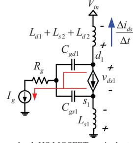
Fig. 13. Synchronous buck HS MOSFET equivalent circuit during  $T_{2f}$
