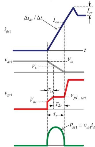
Fig. 7. Synchronous buck HS MOSFET waveforms at turn on with piecewise linear approximations
