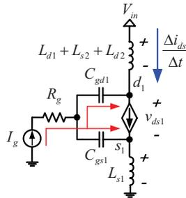
Fig. 8. Synchronous buck HS MOSFET equivalent circuit during  $T_{1r}$
