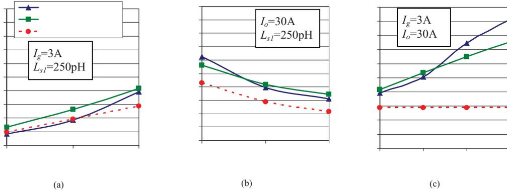
Fig. 14. Total switching loss at 1MHz, 12V input as a function of: (a) load current ( $I_g=3A$ ,  $L_{s1}=250pH$ ), (b) driver supply current ( $I_o=30A$ ,  $L_{s1}=250pH$ ) and (c) common source inductance ( $I_g=3A$ ,  $I_o=30A$ )
