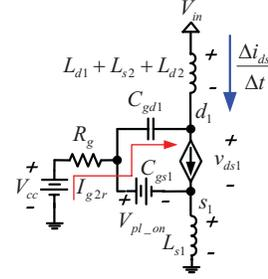
Fig. 9. Synchronous buck HS MOSFET equivalent circuit during  $T_{2r}$ .
