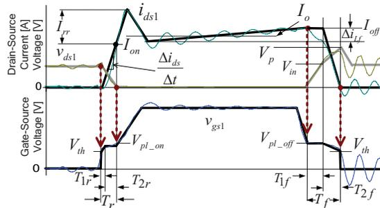
Fig. 6. Synchronous buck HS MOSFET waveforms with piecewise linear approximations of these waveforms in bold
