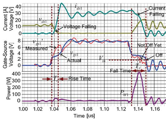
Fig. 2. Synchronous buck voltage regulator HS MOSFET waveforms (top: actual drain-source voltage,  $v_{ds1}$  and drain current,  $i_{ds1}$ ; middle: measured gate-source voltage,  $v_{gs1}$ , and actual gate-source voltage (bold),  $v_{gs1}$ ; bottom: HS MOSFET power,  $v_{ds1}i_{ds1}$ )
