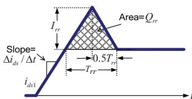
Fig. 10. Synchronous buck HS MOSFET current waveform approximation during reverse recovery at turn on
