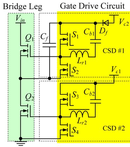
Fig. 9. Bridge leg with the new current-source driver.
