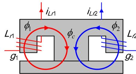
Fig. 11. Integrated inductor structure.
