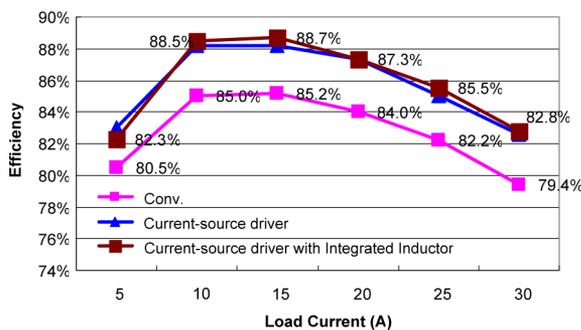
Fig. 18. Efficiency comparison at 1.5 V/30 A/1 MHz.
