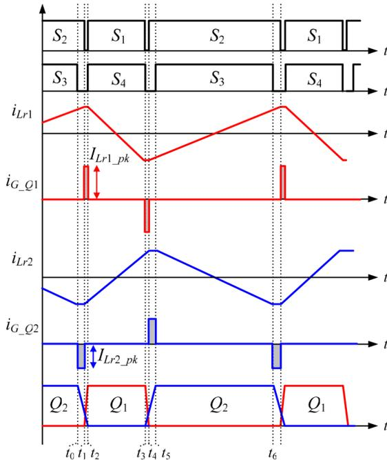
Fig. 4. Key waveforms of the new drive circuit.
