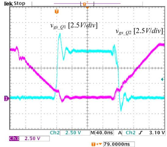
Fig. 14. Gate signals  $v_{gs\_Q1}$  (control FET) and  $v_{gs\_Q2}$  (synchronous FET).
