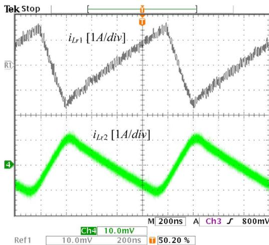
Fig. 17. Waveforms of resonant inductor currents (with magnetic integration).
