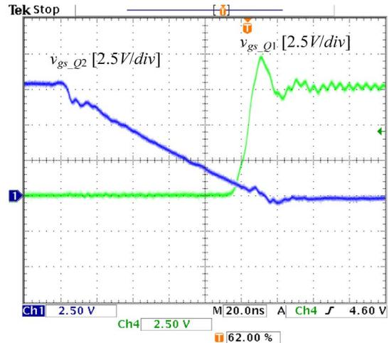
Fig. 15. Zoomed gate signals  $v_{gs\_Q1}$  (control FET) and  $v_{gs\_Q2}$  (synchronous FET).
