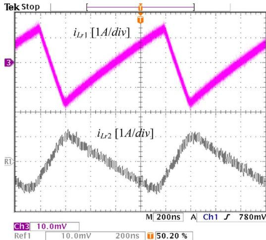
Fig. 16. Waveforms of resonant inductor currents (discrete resonant inductors).
