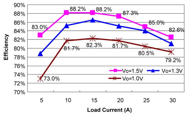
Fig. 20. Efficiency at different output voltages.
