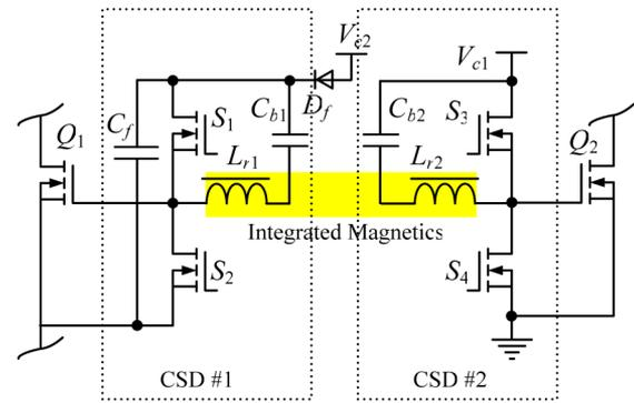
Fig. 10. Proposed current-source driver with integrated inductor.
