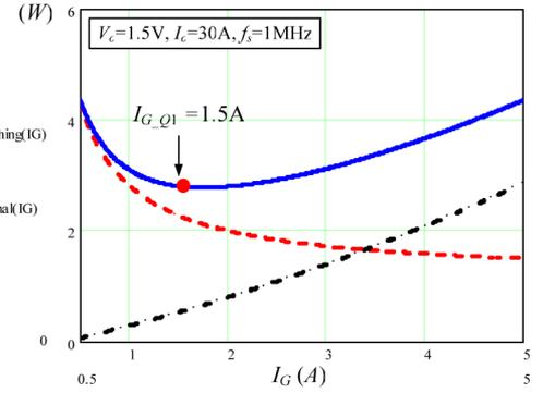
Fig. 6. Optimization curves for the control MOSFET  $Q_1$ : power loss versus gate current.
