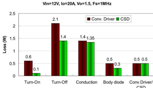
Fig. 8. Loss breakdown between the current-source gate driver and conventional gate driver.
