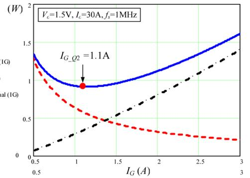
Fig. 7. Optimization curves for the synchronous MOSFET  $Q_2$ : power loss versus gate current.
