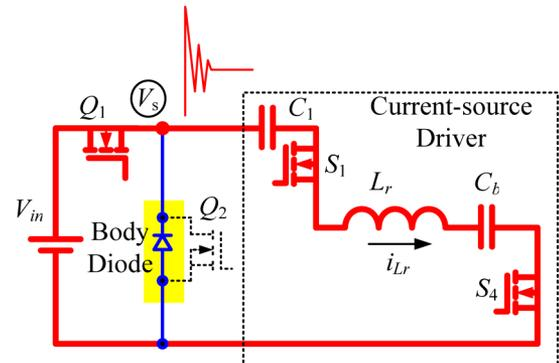
Fig. 2. Equivalent circuit during switching transition.
