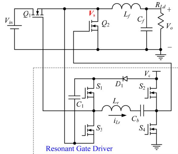
Fig. 1. Buck VR with the resonant gate drive circuit.
