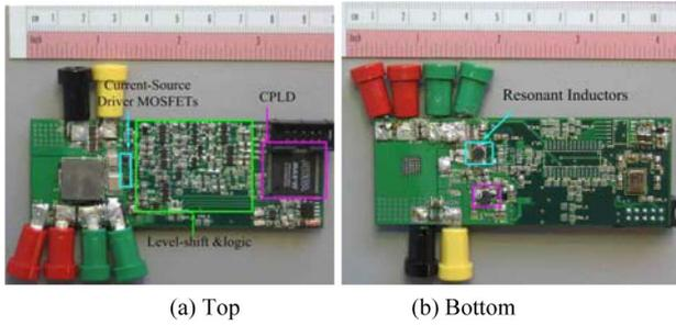
Fig. 13. Prototype photograph of the synchronous buck VR with the proposed current-source gate driver. (a) Top. (b) Bottom.
