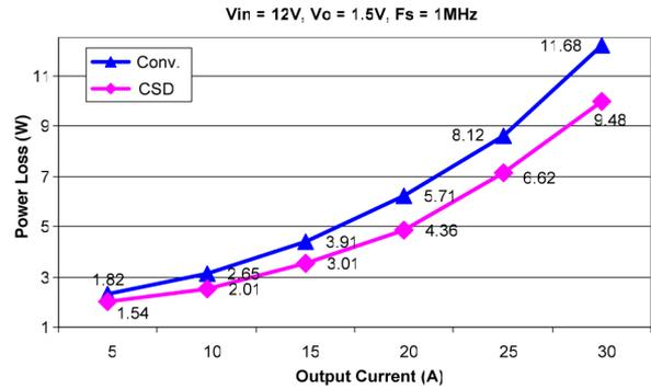
Fig. 19. Power loss comparison at 1.5-V/30-A condition. (Top) Conventional driver (Conv). (Bottom) CSD.
