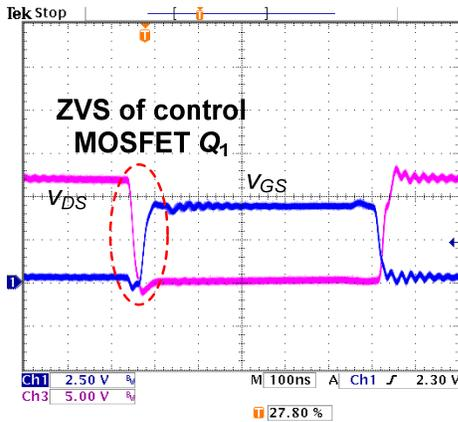
Fig. 8  $v_{DS}$  and  $v_{GS}$  of upper control MOSFET  $Q_1$  @  $I_o=60A$
