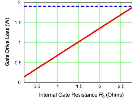
Fig. 5 SR MOSFET gate loss as function of internal mesh resistance  $R_g$
