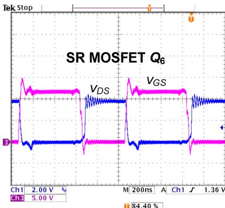
Fig. 10 Gate drive signal and drain-to-source voltage of  $Q_6$  @  $I_o=60A$
