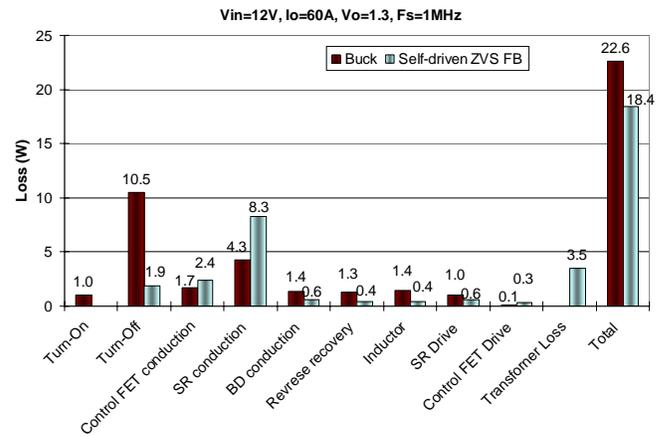
Fig. 6 Loss breakdown comparison
