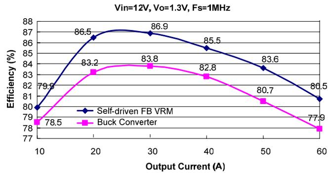
Fig. 11 Efficiency comparison with different load currents:
