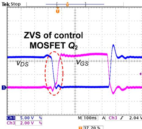
Fig. 9  $v_{DS}$  and  $v_{GS}$  of lower control MOSFET  $Q_2$  @  $I_o=60A$
