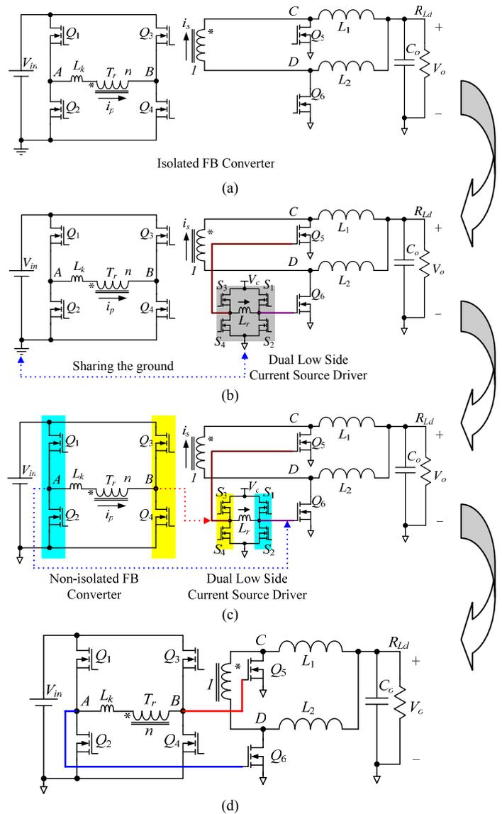
Fig. 1 Proposed ZVS self-driven non-isolated FB converter
