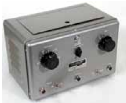
Dr. John Hopps' pacemaker/defibrillator prototype, 1950-1952. Photo courtesy of Canada Science and Technology Museum, Artifact # 1997.0366
