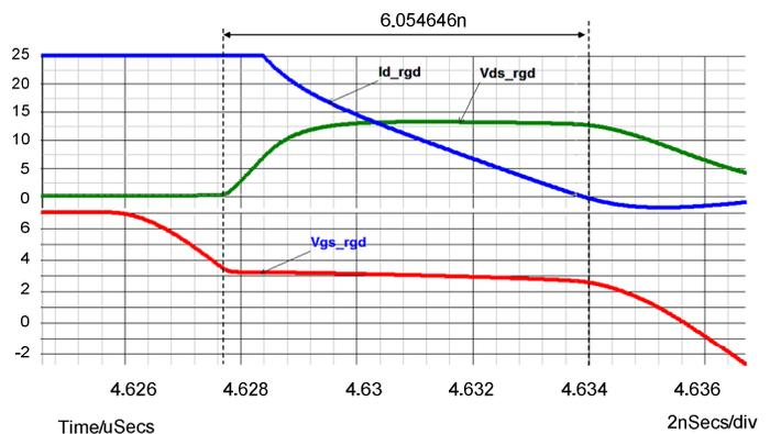
Figure 11 Simulated turn off waveforms of power MOSFET driven by proposed driver
