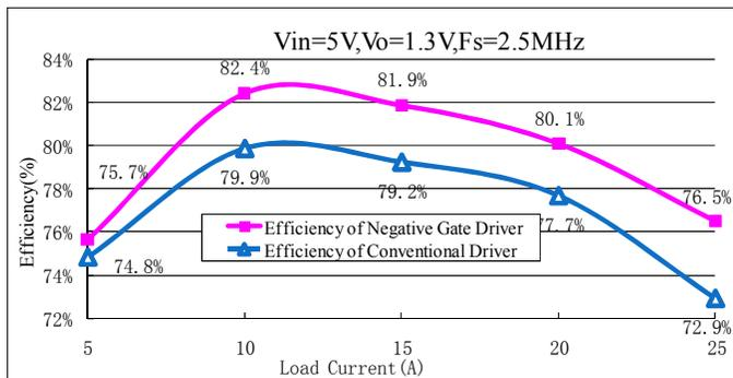
Figure 20 Efficiency comparison at 2.5MHz between proposed driver and conventional driver
