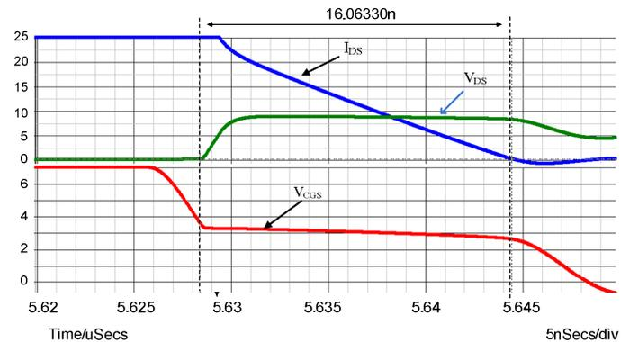
Figure 10 Simulated turn off waveforms of power MOSFET driven by conventional driver
