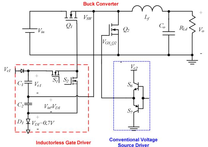
Figure 4 Topology of the proposed inductorless bipolar gate driver
