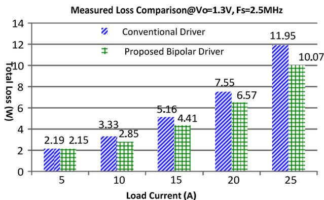
Figure 21 Measured loss comparison at 2.5MHz between proposed driver and conventional driver
