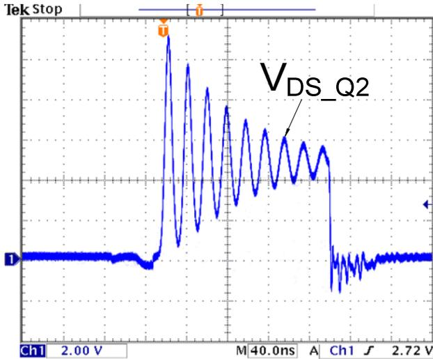
Figure 16 The drain-to-source voltage of Q2:  $V_{DS\_Q2}$
