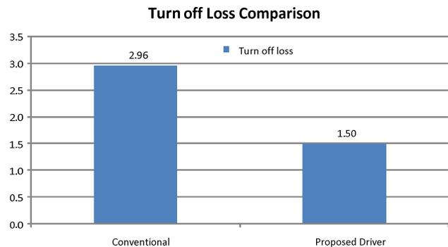
Figure 12 Comparison of the simulated turn-off loss between proposed driver and conventional driver
