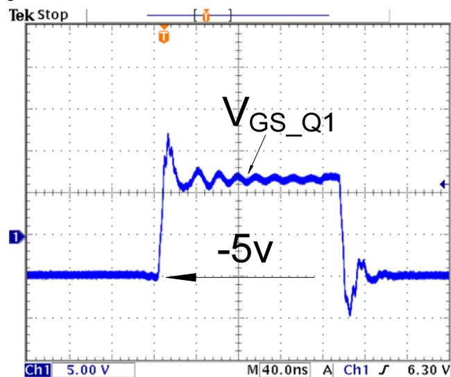
Figure 15 Bipolar Gate Driver signal for  $Q_1$ :  $V_{GS\_Q1}$
