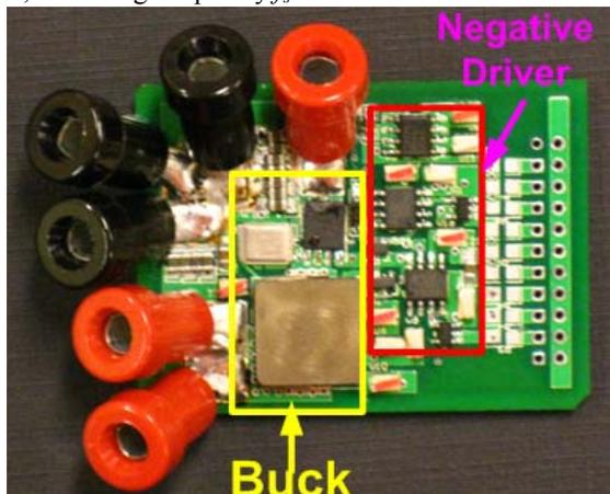
Figure 13 Picture of the synchronous buck converter driven with proposed driver
