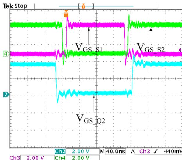
Figure 14 Waveforms of  $V_{GS\_S1}$ ,  $V_{GS\_S2}$ ,  $V_{GS\_Q2}$
