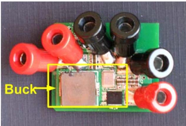
Figure 17 Picture of the buck converter driven with conventional driver
