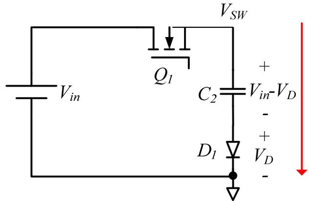
Figure 8 Equivalent circuit for  $C_2$  being charged to  $(V_{IN}-V_{D1})$
