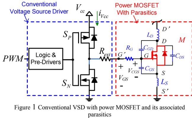
Figure 1 Conventional VSD with power MOSFET and its associated parasitics
