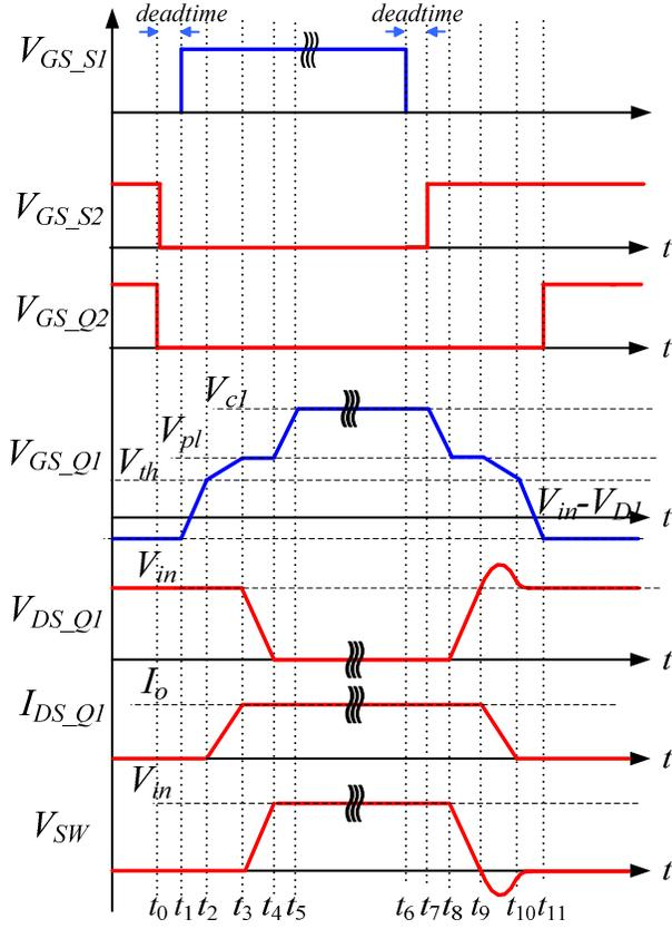
Figure 5 Driver signals and switching waveforms of  $Q_1$
