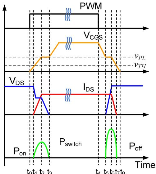
Figure 2 Switching waveforms of power MOSFET driven by the conventional VSD
