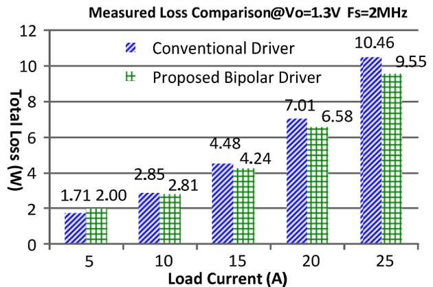
Figure 19 Measured loss comparison at 2MHz between proposed driver and conventional driver
