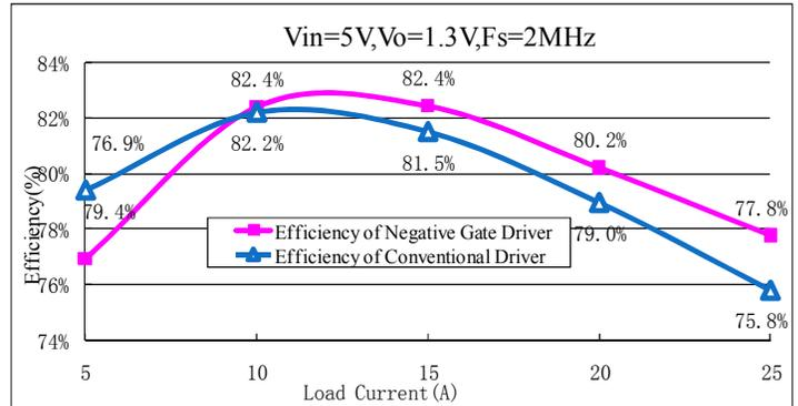
Figure 18 Efficiency comparison at 2MHz between proposed driver and conventional driver
