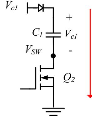
Figure 6 Equivalent circuit for  $C_1$  being charged to  $V_{C1}$
