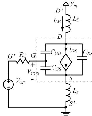
Figure 3 Equivalent circuit of the MOSFET driven by VSD during turn – off transition
