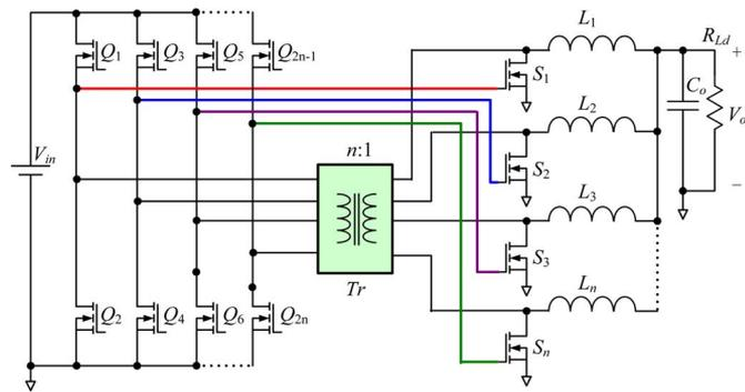
Fig. 11.  $N$ -phase nonisolated ZVS self-driven FB converters with multiple-stage rectifier.
