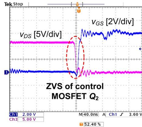
Fig. 13.  $v_{DS}$  and  $v_{GS}$  of  $Q_2$  @  $I_o = 50$  A.
