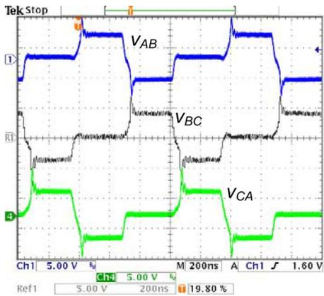
Fig. 15. Secondary-side voltages of transformer at  $I_o = 50$  A.
