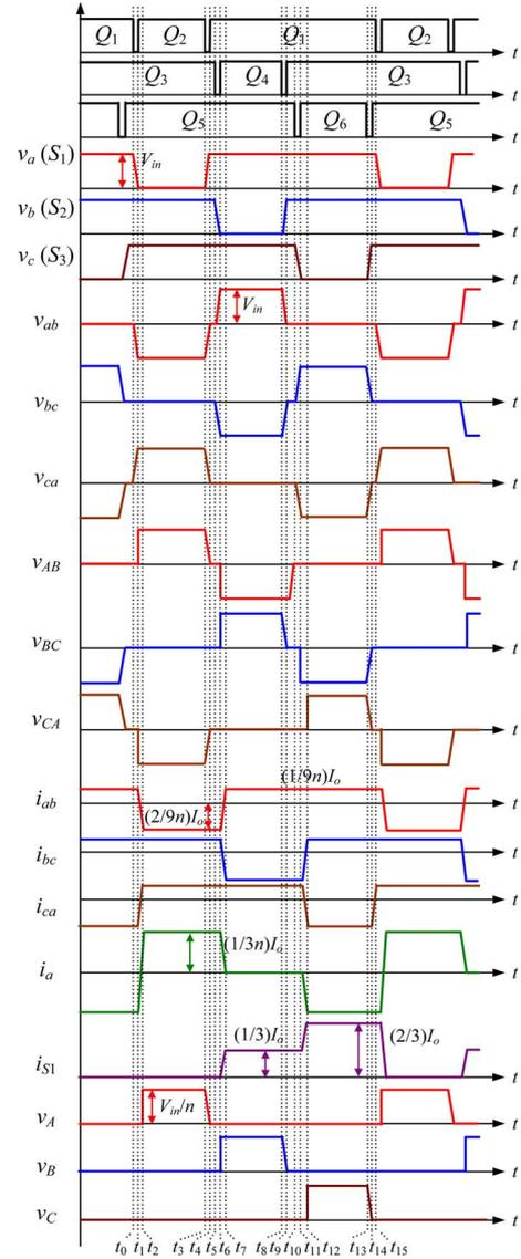
Fig. 2. Key waveforms of the proposed nonisolated current tripler converter.
