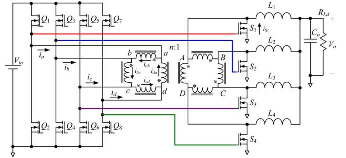
Fig. 8. Proposed four-phase nonisolated ZVS self-driven FB converters.
