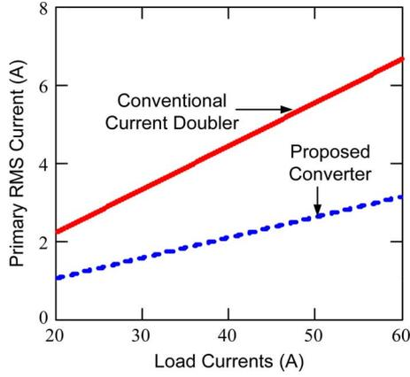
Fig. 6. RMS current comparison of primary windings: Conventional current doubler versus proposed converter.
