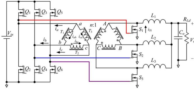
Fig. 1. Proposed nonisolated ZVS self-driven FB converters with current tripler topology.
