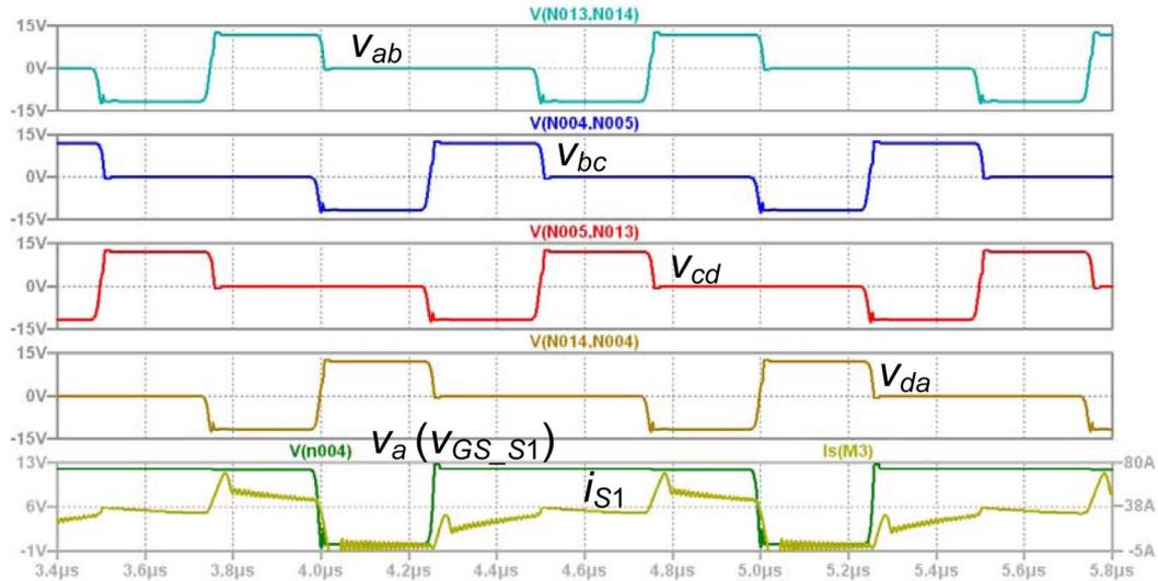
Fig. 10. Simulated waveforms of the self-driven quadrupler rectifier:  $V_{in} = 12$  V,  $V_o = 1.0$  V,  $I_o = 120$  A,  $f_s = 1$  MHz, and  $n = 2$ .
