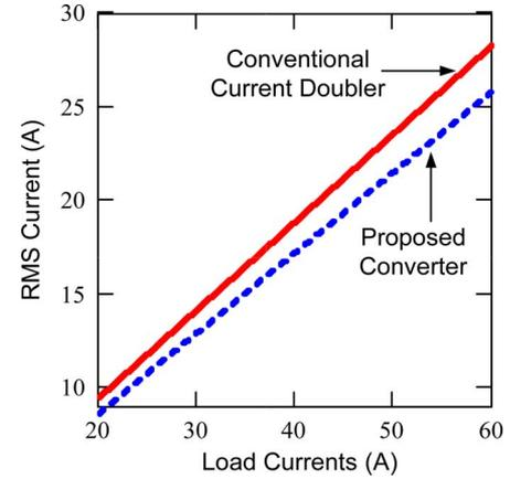
Fig. 4. RMS current comparison of SRs: Conventional current doubler versus proposed converter.
