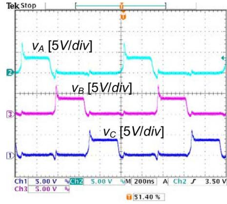
Fig. 17. Rectified voltages at  $I_o = 50$  A.
