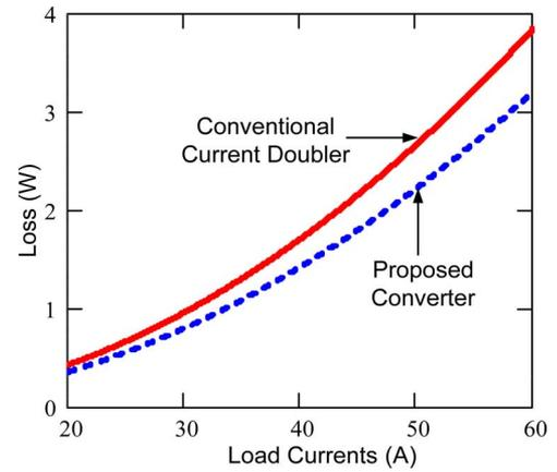
Fig. 5. Conduction loss comparison of SRs: Conventional current doubler versus proposed converter.
