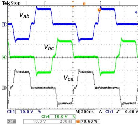
Fig. 14. Primary-side voltages of the transformer at  $I_o = 50$  A.
