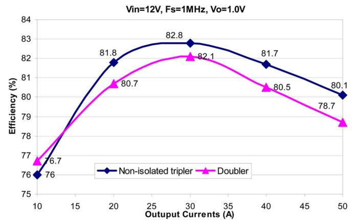
Fig. 18. Efficiency comparison with different load currents. (Top) Nonisolated current tripler. (Bottom) current doubler converter.
