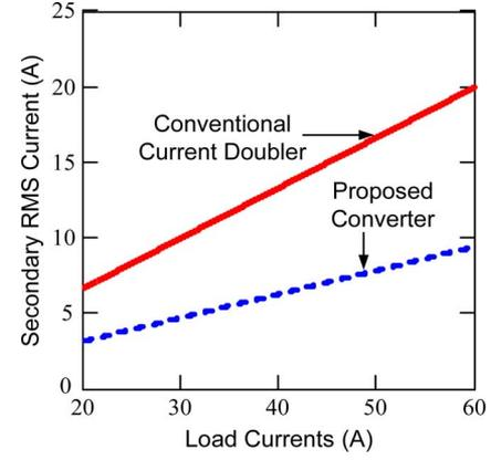
Fig. 7. RMS current comparison of secondary windings: Conventional current doubler versus proposed converter.
