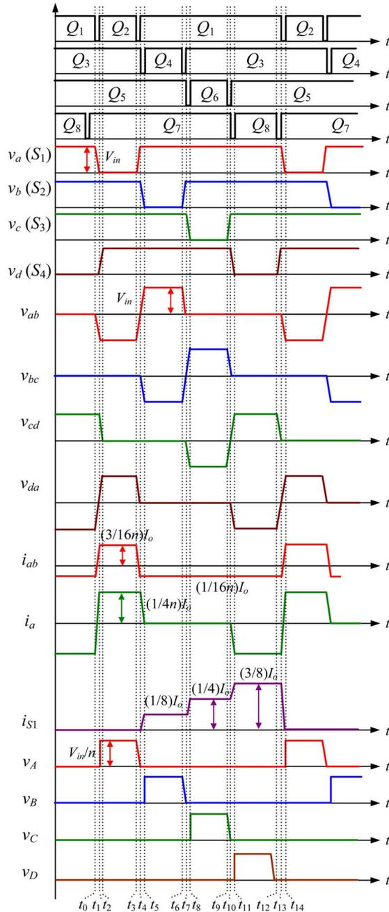
Fig. 9. Key waveforms of four-phase nonisolated ZVS self-driven FB converters with current quadrupler rectifier.
