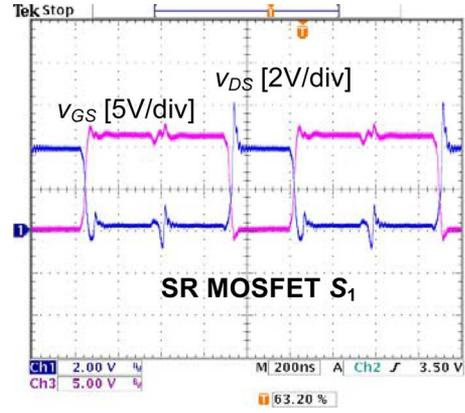
Fig. 16. Gate drive signal and  $v_{DS}$  of SR  $S_1$  at  $I_o = 50$  A.
