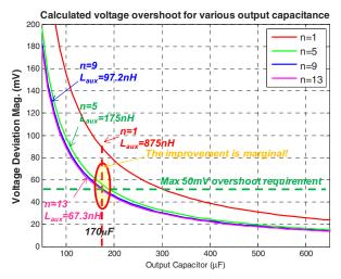
Figure 8 Estimated voltage overshoot for various times of CAC switching and different output capacitance for an unloading transient of 10A ( $V_{in}$ =12V,  $V_o$ =1.5V,  $L_o$ =1uH)
