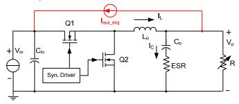
Figure 1 Simplified model of the proposed CAC
