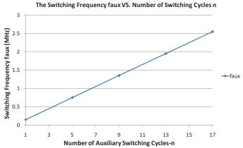
Figure 10 The plot of switching frequency  $f_{aux}$  versus the number *n* of switching cycles
