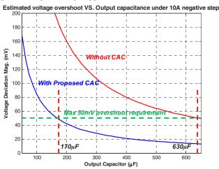
Figure 5 Estimated voltage overshoot for various output capacitance with and without BCM PCM CAC for an unloading transient of 10A ( $V_{in}$ =12V,  $V_o$ =1.5V,  $L_o$ =1uH,  $L_{aac}$ =100nH)
