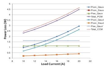
Figure 11 Comparison results of loss breakdown based on different control schemes (the power circuit design parameters:  $V_o=1.5V$ ,  $f_s=450$ kHz,  $L_o=1\mu$ H,  $R_L=1$ m $\Omega$ ,  $L_{aux}=100$ nH,  $RL_{aux}=0.2$ m $\Omega$ ,  $RQ_{aux}=30$ m $\Omega$ ,  $V_{diode}=0.32V$ ,  $T_{fall}=2$ ns)
