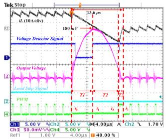
Figure 16 Experimental results of analog CBC controller under 10A ->0A unloading transient without CAC
