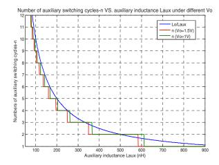
Figure 6 Number of auxiliary switching cycles n (as well as the ratio of  $L_o/L_{aux}$ ) and the auxiliary inductance value under different output voltages  $V_o$
