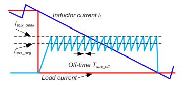
Figure 3 Peak current mode, constant off-time operation of the proposed controller
