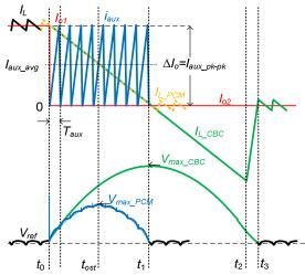
Figure 4 BCM Peak current mode (PCM) CAC and normal CBC operation waveforms
