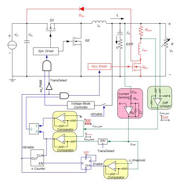
Figure 13 Hardware implementation of the proposed BCM PCM CAC
