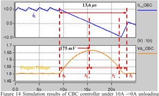
Figure 14 Simulation results of CBC controller under 10A ->0A unloading transient without CAC for a single phase Buck converter
