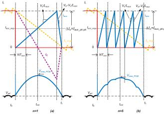
Figure 9 Controlled auxiliary current switching for n cycles by selecting different  $L_{aux}$  (a)n=1,  $L_{aux}$ =875nH; (b)n=5,  $L_{aux}$ =175nH ( $V_{in}$ =12V,  $V_o$ =1.5V,  $L_o$ =1uH)
