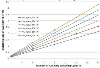
Figure 12 The plot of switching loss of the auxiliary FET versus the number n of auxiliary switching cycles under various load step unloading transients (the power circuit design parameters:  $V_o = V_{ref} = 1.5 \text{ V}$ ,  $f_s = 450 \text{ kHz}$ ,  $T_{fall} = 2 \text{ ns}$ )
