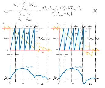
Figure 7 The effect of rounding down operation of n on the settling time, (a)  $[(V_{in}-V_o)/V_{in}*L_o/L_{aux}]$ -n $\leq$ 0.5;(b)  $[(V_{in}-V_o)/V_{in}*L_o/L_{aux}]$ -n $\geq$ 0.5
