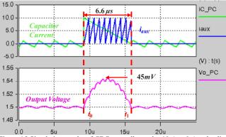
Figure 15 Simulation results of CBC controller under 10 A ->0 A unloading transient with proposed CAC for a single phase Buck converter
