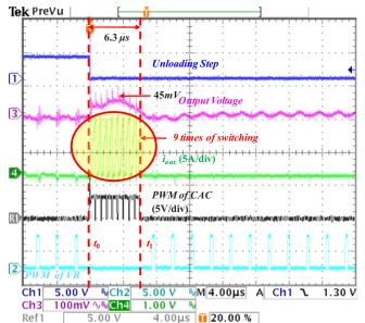
Figure 17 Experimental results of the proposed BCM PCM controller under 10A ->0A unloading transient with CAC
