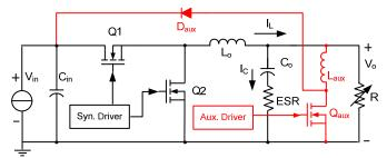
Figure 2 MOSFET-diode implementation of the CAC
