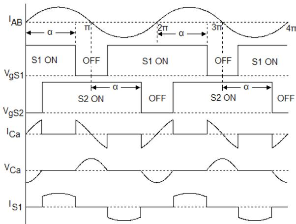
Figure 2 Waveforms of SCC.
