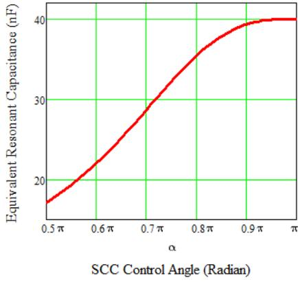
Figure 6 SCC Control Angle VS. Equivalent Resonant Capacitance.
