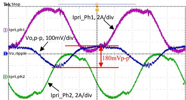
Figure 12 Output voltage ripple,  $I_o=50A$ , two-phase interleaved SCC-LLC.
