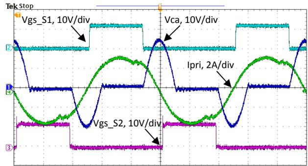
Figure 9 SCC operation,  $I_o=20A$ ,  $\alpha=131^\circ$ .
