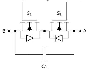
Figure 1 Structure of SCC.
