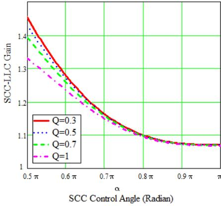
Figure 7 SCC Control Angle VS. SCC-LLC Gain.
