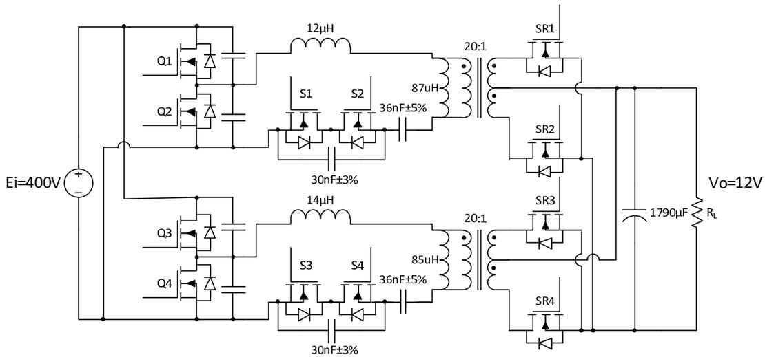
Figure 8 The implemented two-phase interleaved SCC-LLC.
