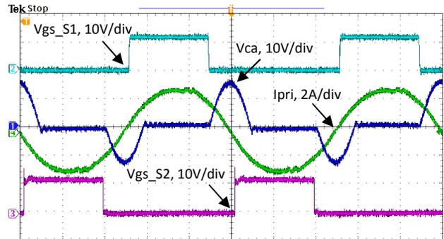
Figure 10 SCC operation,  $I_o=10A$ ,  $\alpha=136^\circ$ .
