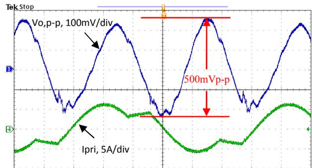
Figure 11 Output voltage ripple,  $I_o=50A$ , single phase LLC.
