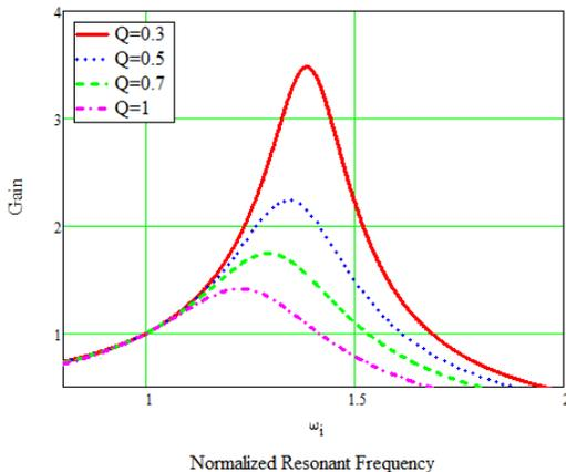
Figure 5 Gain plot, varying  $Q$ .
