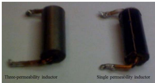
Fig. 12. Pictures of the inductor prototypes.
