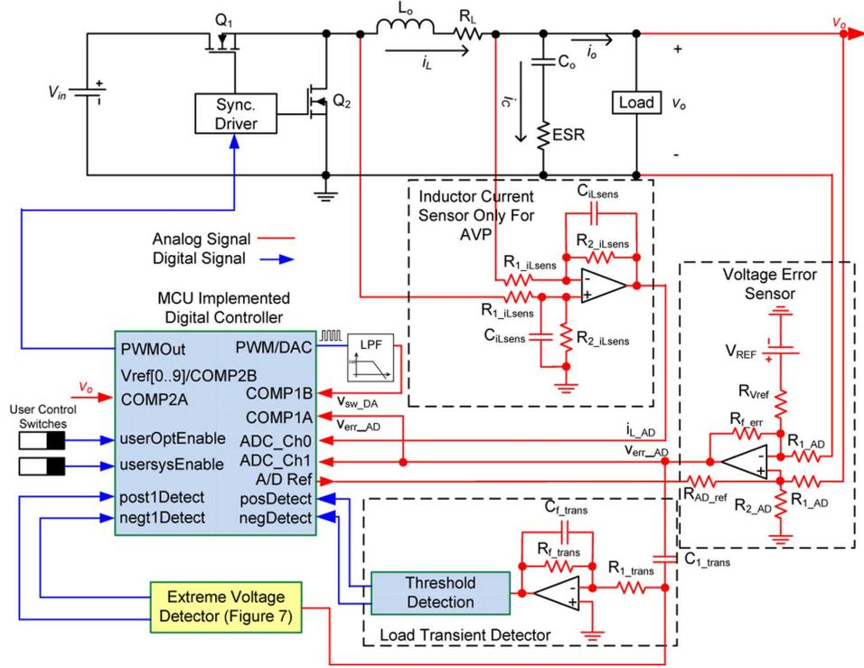
Fig. 5. Hardware implementation diagram of the digital control system.
