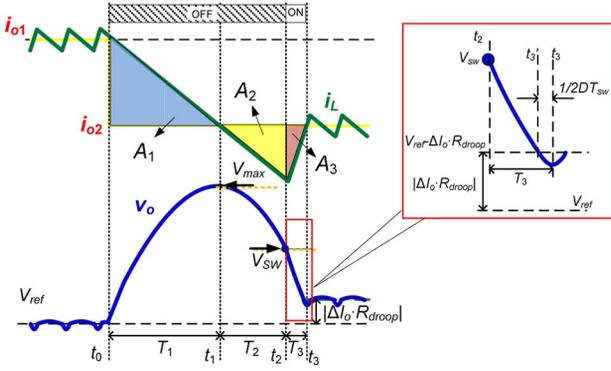
Fig. 4. Inductor current and capacitor voltage waveforms for AVP applications under unloading step transient case ( $R_{droop}$ : droop resistance).
