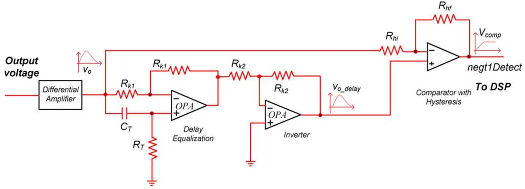
Fig. 7. Hardware implementation of the detector based on the adjustable delay circuit.
