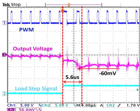
Fig. 15. Experimental result of 10 A loading step transients under AVP operation using proposed V- CBC controller.
