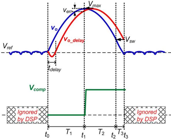
Fig. 6. Illustration of the proposed analog extreme voltage detector under unloading step transient case for  $t_1$  detection and  $V_{max}$  sensing.
