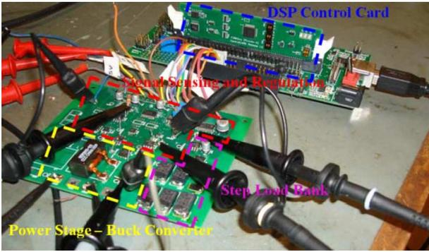
Fig. 10. Experimental prototype of the proposed V-CBC controlled dc-dc Buck converter.
