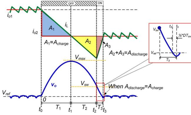
Fig. 1. Capacitor charge integral areas during an unloading step transient.
