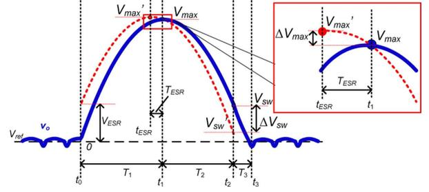
Fig. 3. Impact of output capacitor  $ESR$  on the output voltage.
