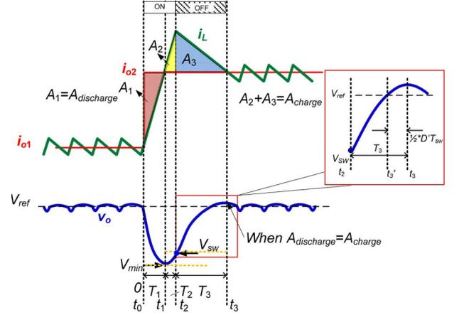
Fig. 2. Capacitor charge integral areas during a loading step transient.
