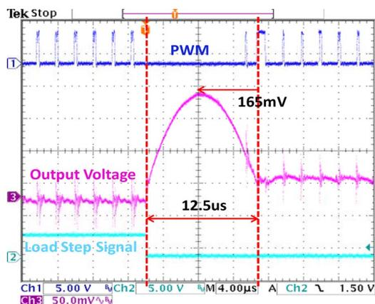
Fig. 16. Experimental result of 10 A unloading step transients under AVP using proposed V- CBC controller.
