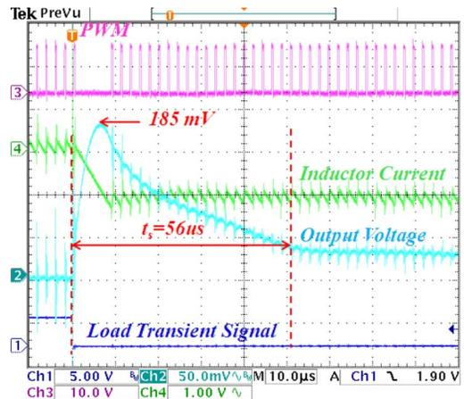
Fig. 13. Experimental results of Buck converter under unloading step transient case 10 A- 0 A using linear mode controller.
