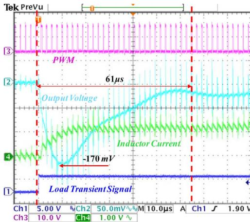
Fig. 11. Experimental results of Buck converter under loading step transient case 0 A- 10 A using linear mode controller.
