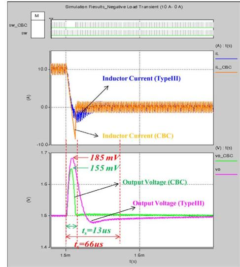
Fig. 9. Simulation results of unloading transient case for comparison between V-CBC and linear mode of controller (10 A → 0 A).
