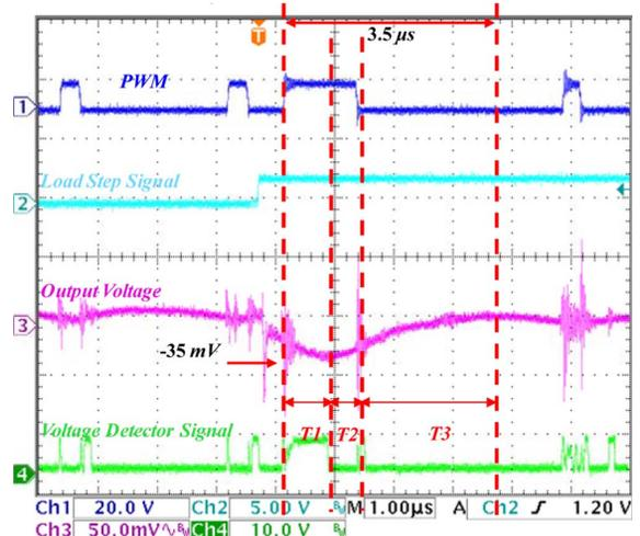
Fig. 12. Experimental results of Buck converter under loading step transient case 0 A- 10 A using V-CBC controller.
