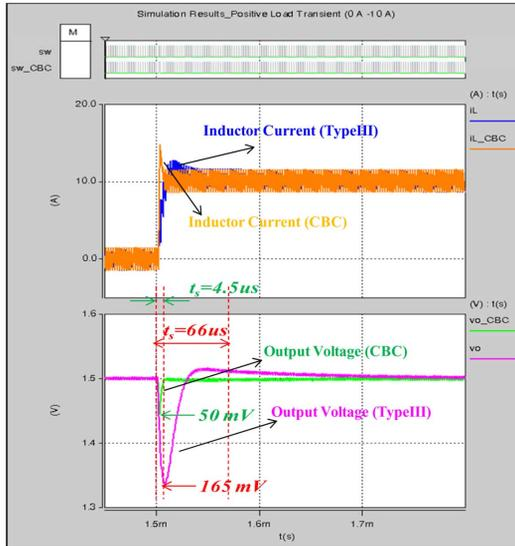
Fig. 8. Simulation results of loading step transient case for comparison between V-CBC and linear mode of controller (0 A → 10 A).
