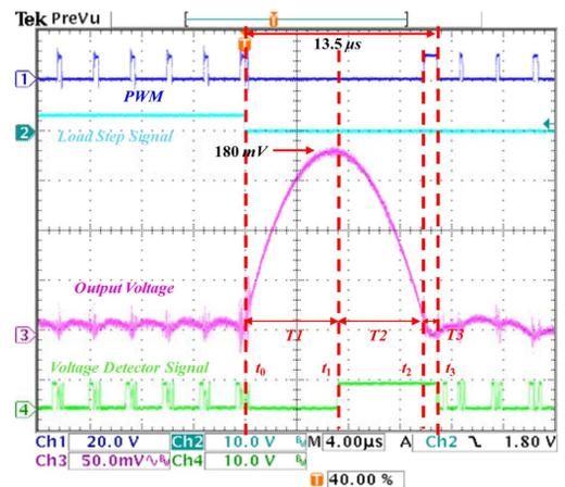
Fig. 14. Experimental results of Buck converter under unloading step transient case 10 A- 0 A using V-CBC controller.
