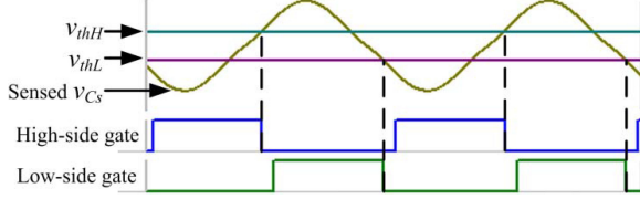
Fig. 2. Operation waveforms of a BBCC-controlled LLC converter.
