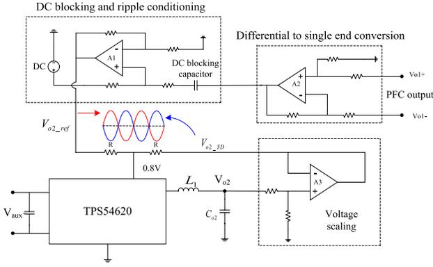
Fig. 8. Detailed circuit implementation of the RCC.
