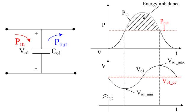
Fig. 5. Energy imbalance between input and output and the resulted  $V_{o1}$  ripple.
