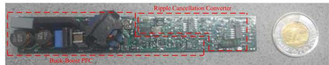
Fig. 22. Photo of the Buck-Boost experimental prototype.
