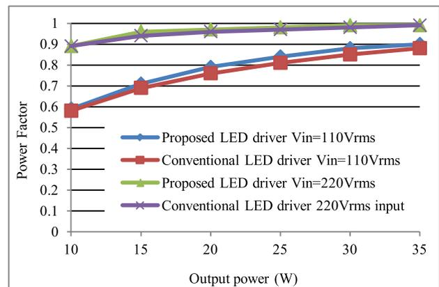
Fig. 14. Power factor of the proposed LED driver and the conventional LED driver.
