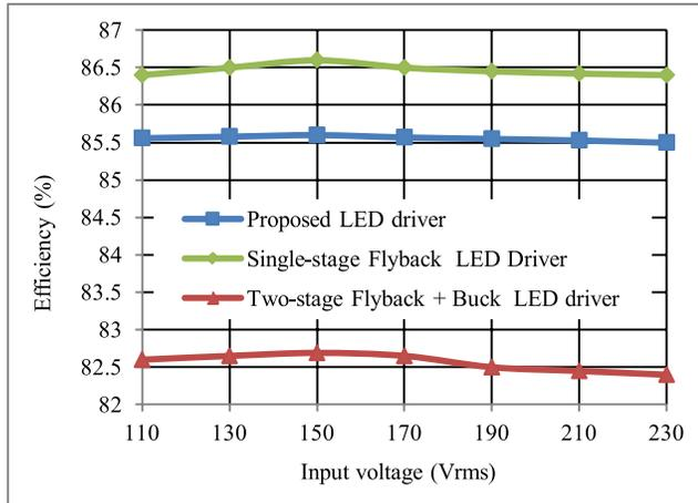
Fig. 16. Efficiency comparison between different designs at full load (50 V/0.7 A).
