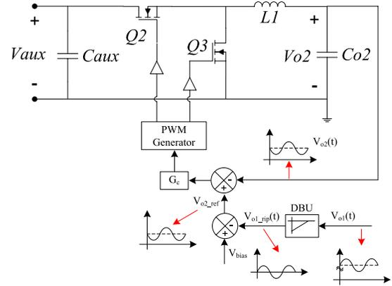
Fig. 7. Control diagram of the RCC.
