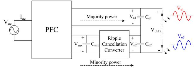
Fig. 1. Generic power stage structure of the proposed ripple cancellation LED driver.
