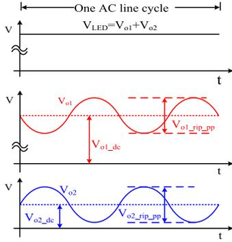
Fig. 3. Critical waveforms of the proposed LED driver.
