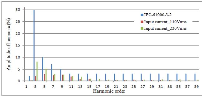
Fig. 15. Measured harmonic content of the input current.
