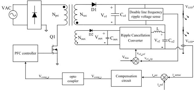
Fig. 9. Control diagram of the proposed Flyback ripple cancellation LED driver.
