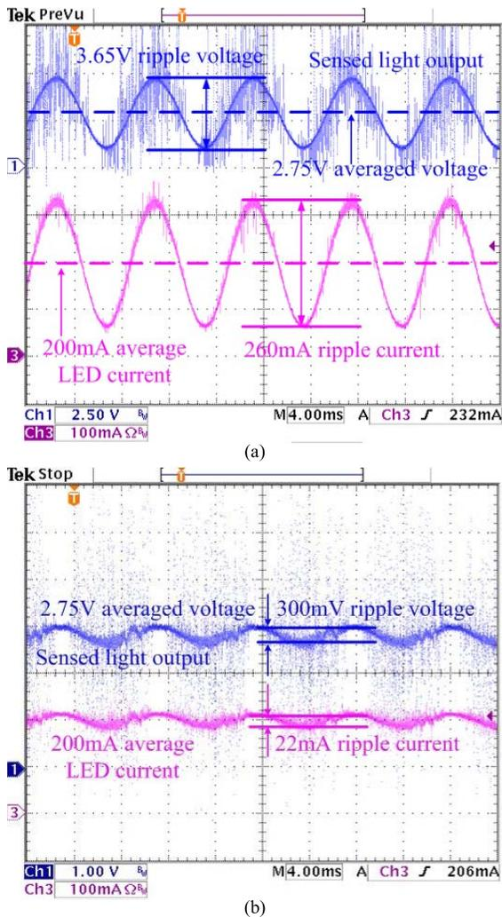
Fig. 20. Ripple current and light flickering comparison between the proposed LED driver and the conventional LED driver. (a) Conventional Buck-Boost LED driver. (b) Proposed Buck-Boost LED driver.
