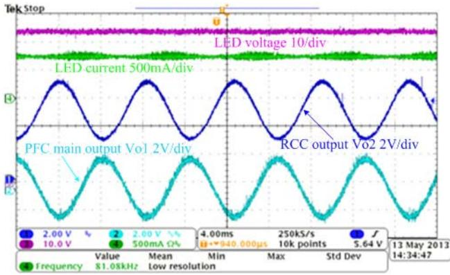
Fig. 11. Key waveforms of the proposed Flyback LED driver prototype ( $V_{in} = 110 V_{rms}$ ,  $V_{LED} = 50 V$ , and  $I_{LED} = 0.7 A$ ).
