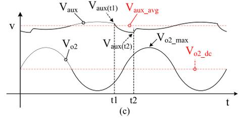
Fig. 10. Design consideration for  $C_{aux}$ . (a) Waveform of the input power and the required power to maintain  $V_{o2}$ . (b) Zoomed-in-view of (a). (c) Relationship of the waveform  $V_{aux}$  and  $V_{o2}$ .
