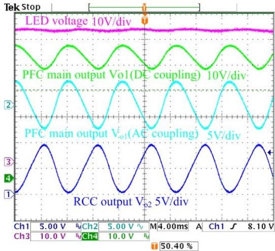
Fig. 19. Key waveforms of the proposed Buck-Boost LED driver ( $V_{in} = 110$  V<sub>rms</sub>,  $V_{LED} = 50$  V, and  $I_{LED} = 0.2$  A).
