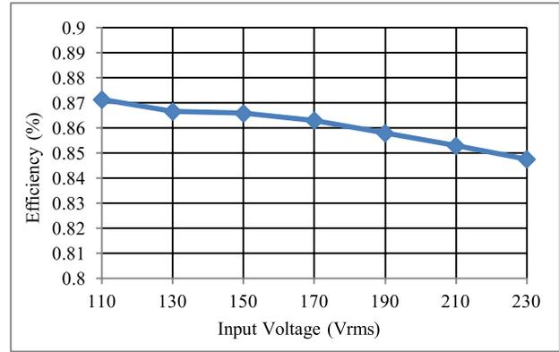
Fig. 21. Efficiency of the Buck-Boost experimental prototype at full load (50 V/0.2 A).
