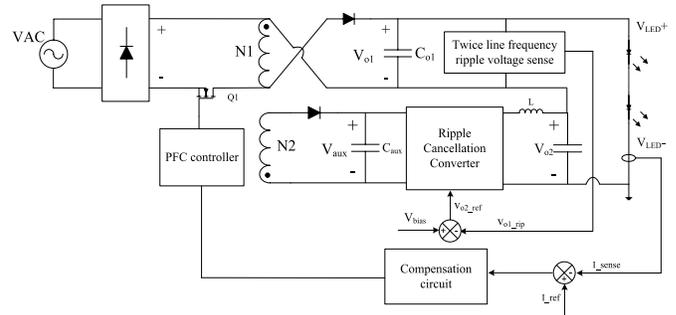
Fig. 18. Circuit diagram of the proposed Buck-Boost LED driver prototype.
