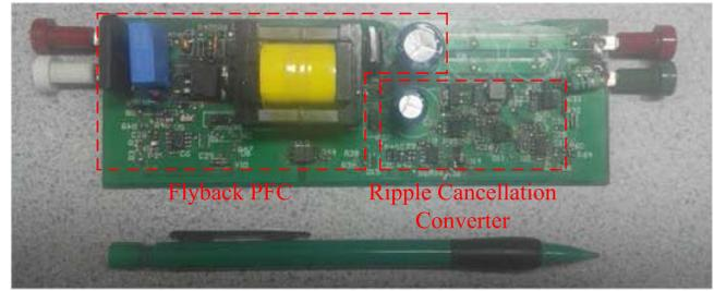
Fig. 17. Photo of the Flyback experimental prototype.
