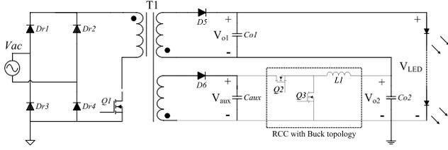
Fig. 2. Power stage of the proposed Flyback-based ripple cancellation LED driver.
