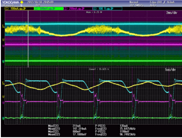
Fig. 19. Experimental results at light load (CH1-Yellow: fan current; CH2-Green: V_{\text{ramp}} ; CH3-Pink: I_{Q1} ; CH4-Blue: V_{ds} of Q1).
