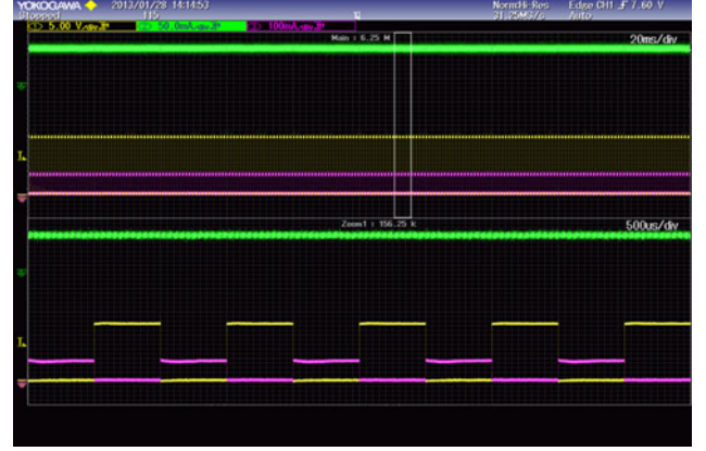
Fig. 21. Transient performance during AUX load changes at 1 kHz (CH1-Yellow: control switch voltage of the auxiliary load, CH2-Green: load current at 70 mA, CH3-Pink: auxiliary load current, 1.2-W resistive load + 1.8-W fan load).
