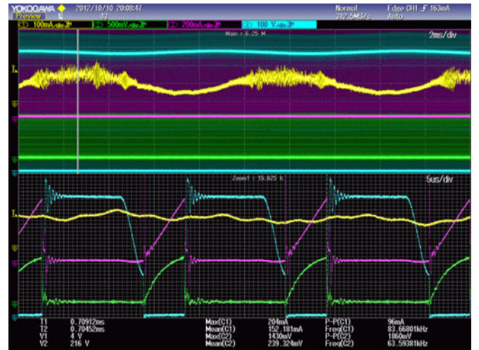
Fig. 18. Experimental results at full load (CH1-Yellow: fan current; CH2-Green: V_{ramp} ; CH3-Pink: I_{Q1} ; CH4-Blue: V_{ds} of Q1).
