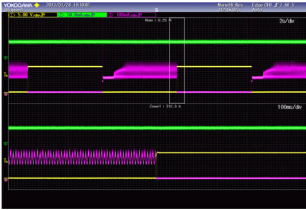
Fig. 20. Transient performance during AUX load changes at 0.1 Hz (CH1-Yellow: control switch voltage of the auxiliary load, CH2-Green: load current at 70 mA, CH3-Pink: auxiliary load current, 1.2-W resistive load + 1.8-W fan load).
