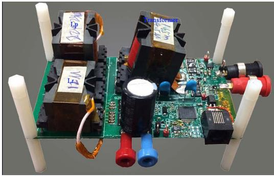
Fig. 10. Prototype of the 250 – 400V input 12V/500W output LCLC resonant converter
