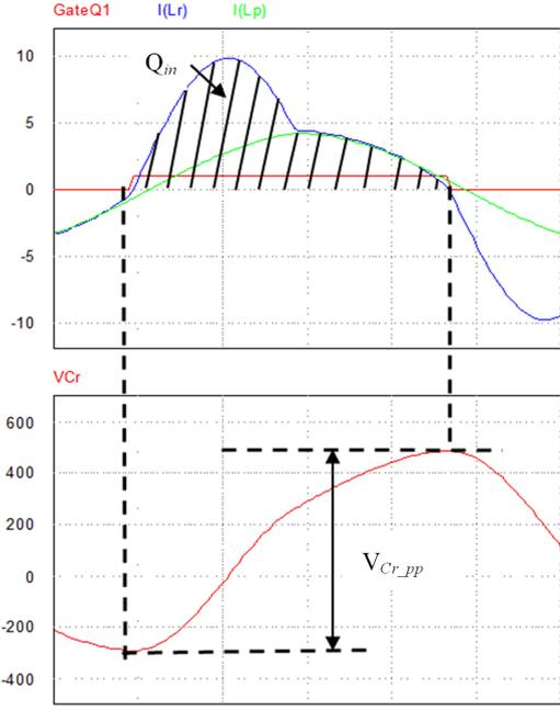
Fig. 12.  $C_r$  charging waveform at minimum frequency.
