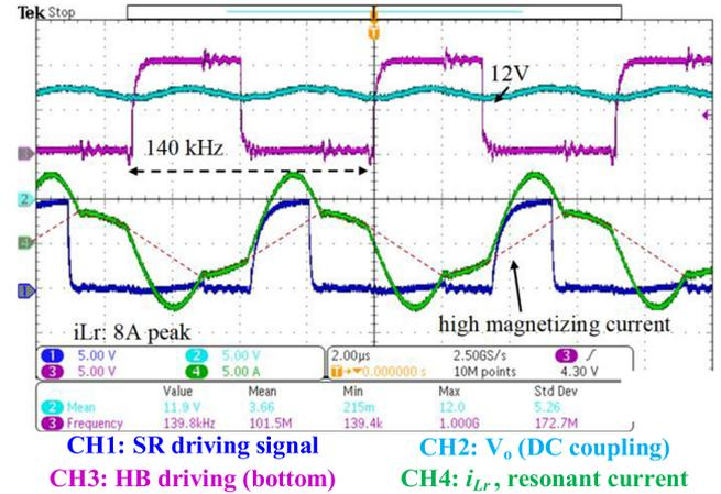
Fig. 15. 250 V input, 12 V/40 A output steady-state waveform.
