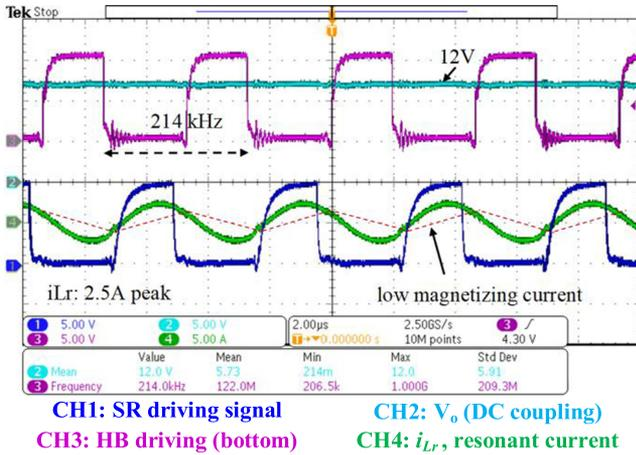
Fig. 17. 400 V input, 12 V/20 A output steady-state waveform.
