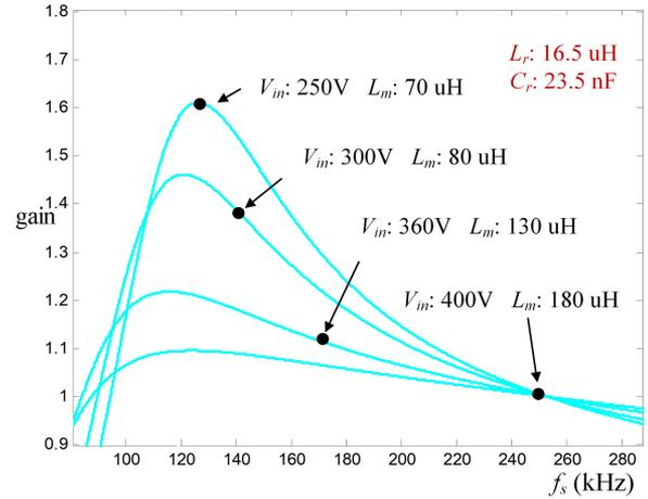
Fig. 3. Desired *LLC* with different  $L_m$  for hold-up operation ( $L_r = 16.5 \mu\text{H}$ ,  $C_r = 23.5 \text{ nF}$ ).
