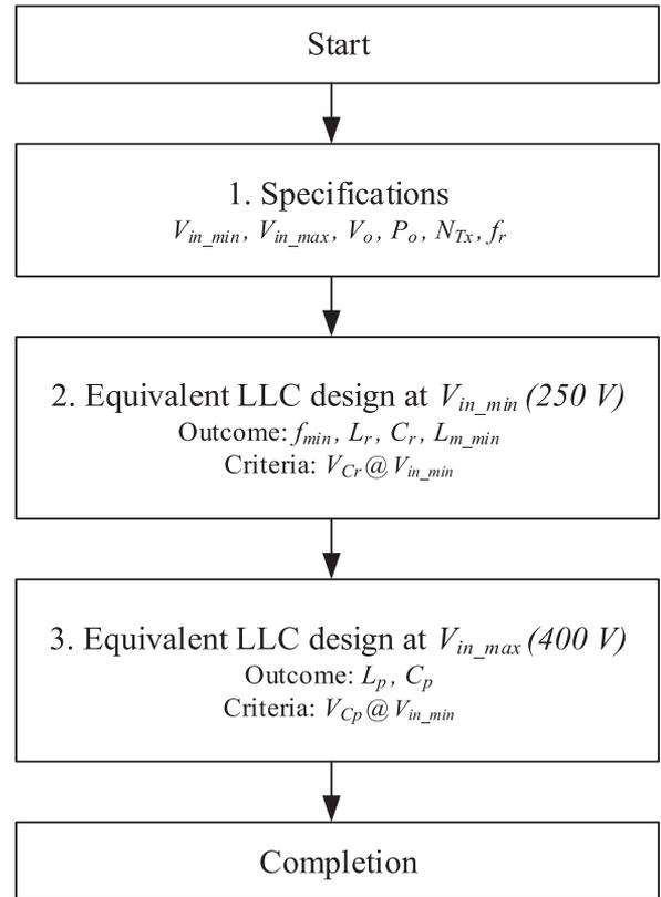
Fig. 11. Design flowchart of the proposed design method based on capacitor voltage stress.
