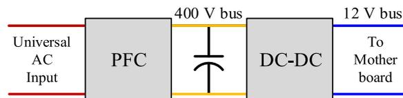
Fig. 1. Structure of the front-end converter.
