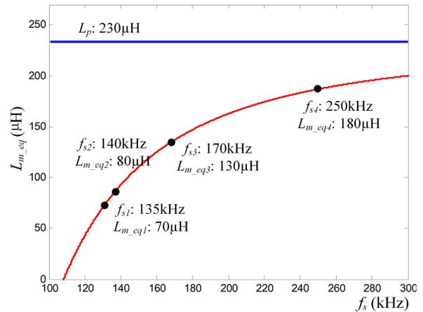
Fig. 4. Equivalent  $L_{m\_eq}$  changing with  $f_s$  ( $L_p = 230 \mu\text{H}$ ,  $C_p = 9.4 \text{ nF}$ ).
