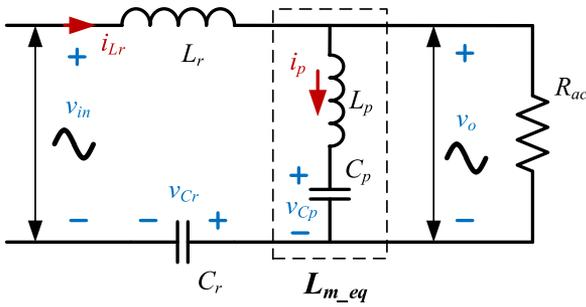
Fig. 6. First harmonic approximation of *LCLC* converter.
