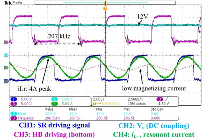
Fig. 14. 400 V input, 12 V/40 A output steady-state waveform.
