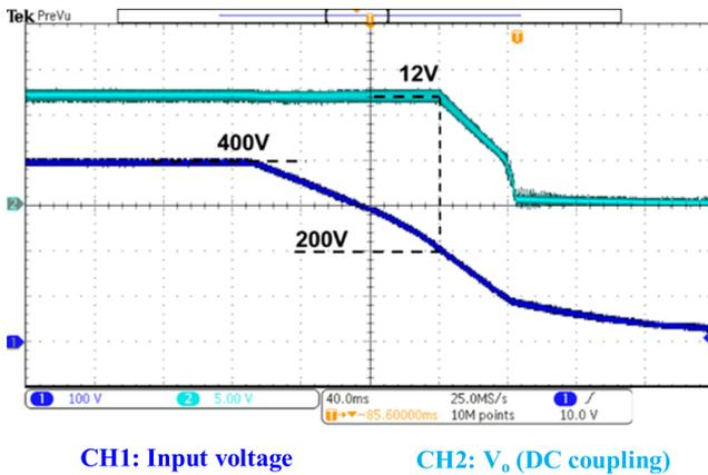
Fig. 19. Hold-up test under half load.
