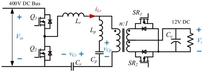
Fig. 5. *LCLC* converter topology with center tapped transformer and SR.
