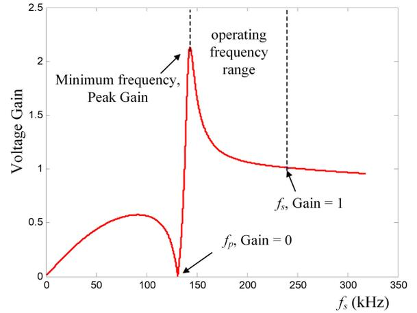
Fig. 7. Typical gain curve of *LCLC* converter.
