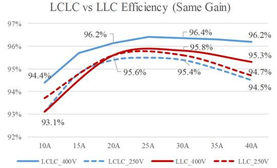
Fig. 20. Efficiency comparison of *LCLC* and *LLC* for 250 and 400 V.
