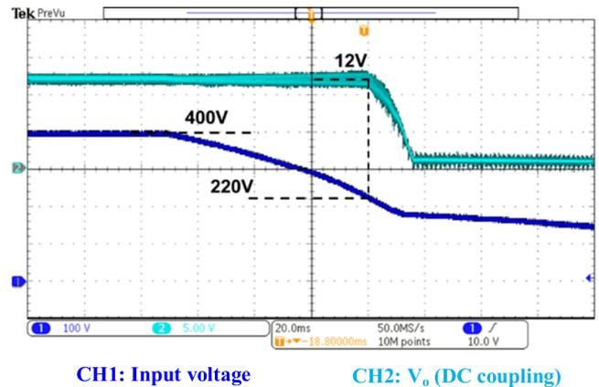
Fig. 16. Hold-up test under full load.
