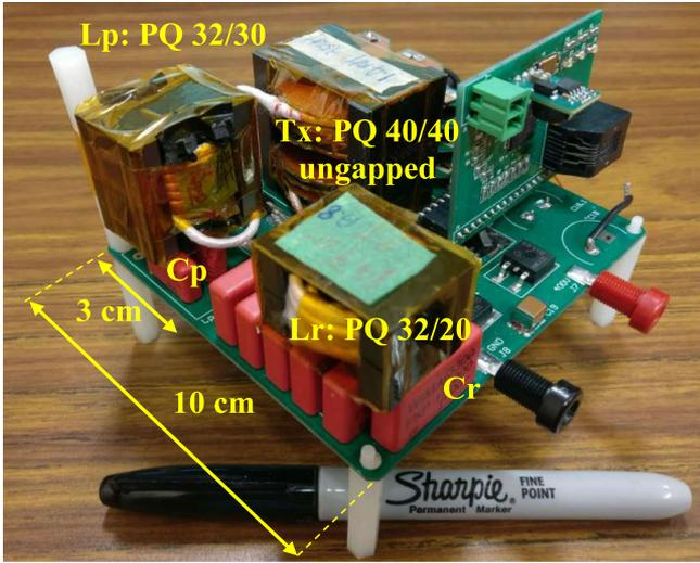
Fig. 13. Picture of the prototype.
