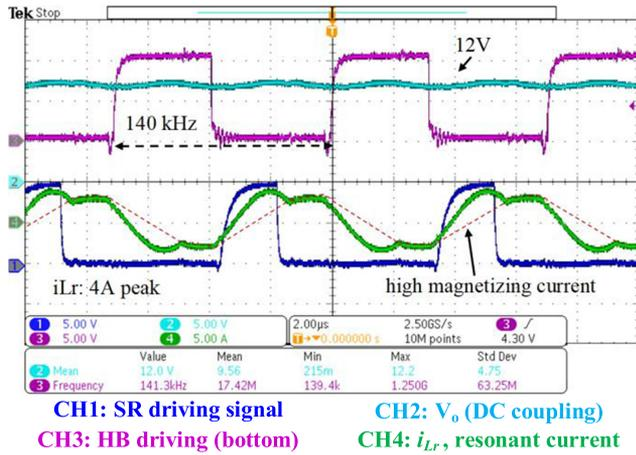
Fig. 18. 250 V input, 12 V/20 A output steady-state waveform.
