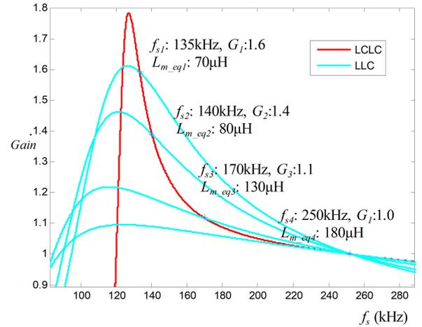
Fig. 8. *LCLC* gain curve fits the *LLC* gain curves at specific operating points ( $L_r = 16.5 \mu\text{H}$ ,  $C_r = 23.5 \text{ nF}$ ,  $L_p = 230 \mu\text{H}$ ,  $C_p = 9.4 \text{ nF}$ ).
