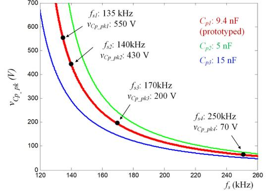
Fig. 10. Voltage stress on  $C_p$  at different switching frequencies.
