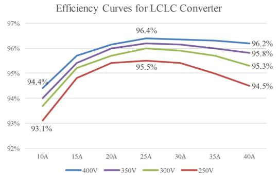
Fig. 21. Efficiency curves of different input voltage level versus load.
