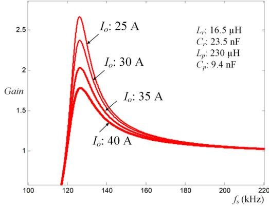
Fig. 9. LCLC gain curve at different load condition.
