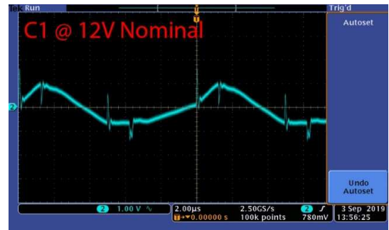
Figure 15: Voltage waveform of flying capacitor C1 at full load. Using capacitors as designed in Table 3.
