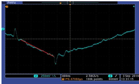
Figure 9: Magnified voltage waveform of C3, centered around the instance where it is carrying full load current.
