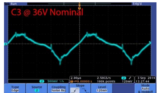
Figure 17: Voltage waveform of flying capacitor C3 at full load. Using capacitors as designed in Table 3.
