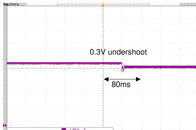
Fig. 20. Output voltage waveforms of 5 V for load step of 1 to 20 A.
