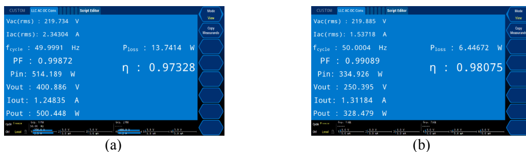
Fig. 9. Efficiency measurement results with the proposed synchronous rectification strategy for (a) V_o=400 V, P_o=500 W, and (b) V_o=250 V, P_o=330 W.
