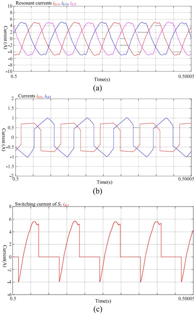
Fig. 6. Simulated waveforms of the proposed multioutput converter at  $V_{out} = 300$  V,  $V_{aux1} = 36$  V, and  $V_{aux2} = 48$  V with a full load. (a) Resonant currents of the three-phase resonant tank. (b) Currents of the full-bridge converter. (c) Switching current of the power switch  $S_1$ .
