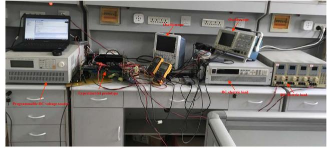
Fig. 8. Experimental platform of the proposed converter.
