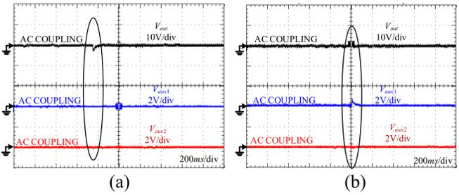
Fig. 12. Measured load transient waveforms:  $P_{aux1}$  switches from half power to full power with  $P_{out}$  and  $P_{aux2}$  remain unchanged; time scale:  $200$  ms/div.
