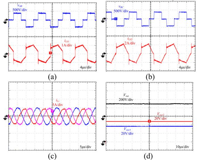
Fig. 9. Experimental waveforms at  $V_{out} = 300$  V,  $V_{aux1} = 36$  V, and  $V_{aux2} = 48$  V with a full load. (a) Measured current waveforms of the full-bridge converter  $V_{aux1}$ . (b) Measured current waveforms of the full-bridge converter  $V_{aux2}$ . (c) Resonant currents of the three-phase resonant tank  $i_{Lr1}$ ,  $i_{Lr2}$ , and  $i_{Lr3}$ . (d) Measured output voltages  $V_{out}$ ,  $V_{aux1}$ , and  $V_{aux2}$ .
