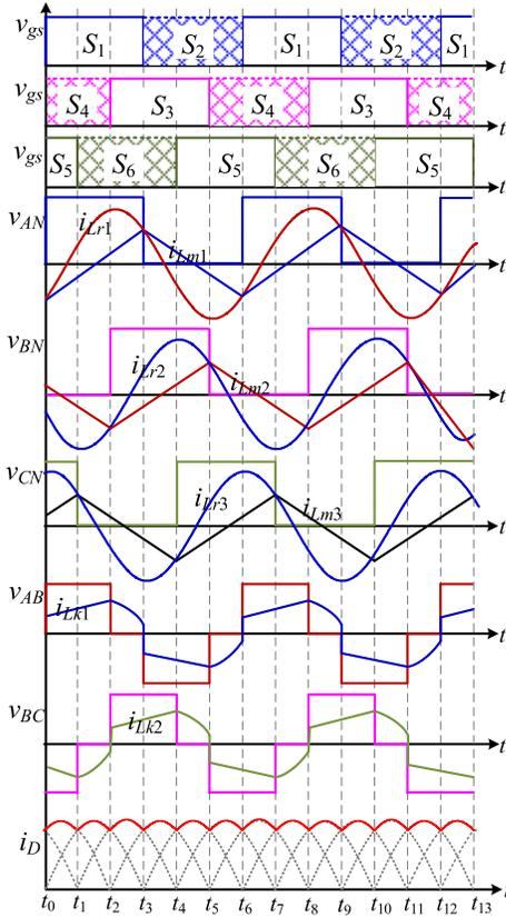
Fig. 4. Principal waveforms of the proposed converter.
