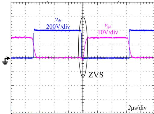
Fig. 11. Switching voltage and gate-driving signal; time scale:  $2 \mu\text{s}/\text{div}$ .
