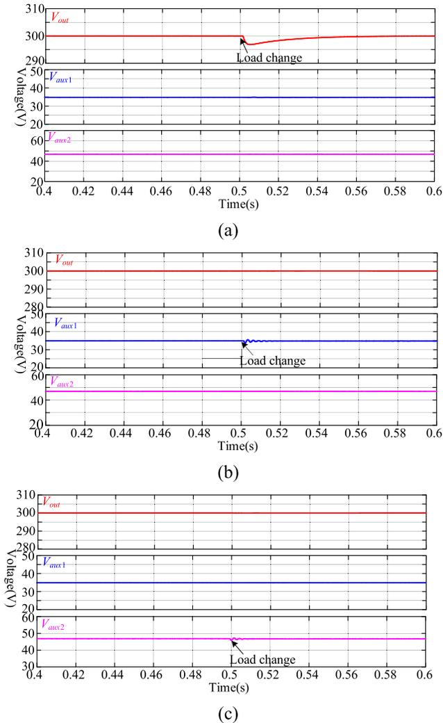
Fig. 7. Transient waveforms ( $V_{out} = 300$  V,  $V_{aux1} = 36$  V, and  $V_{aux2} = 48$  V). (a)  $P_{out}$  switches from half power to full power with  $P_{aux1}$  and  $P_{aux2}$  remain unchanged. (b)  $P_{aux1}$  switches from half power to full power with  $P_{out}$  and  $P_{aux2}$  remain unchanged. (c)  $P_{aux2}$  switches from half power to full power with  $P_{out}$  and  $P_{aux1}$  remain unchanged.
