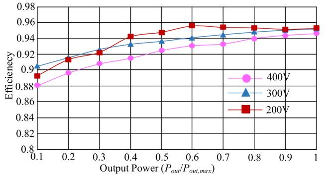
Fig. 13. Efficiency versus output power ( $P_{aux1} = 200$  W and  $P_{aux2} = 200$  W).
