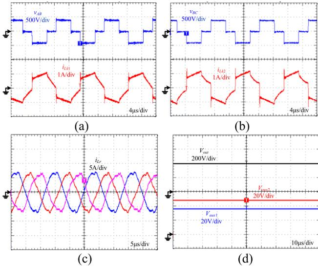
Fig. 10. Experimental waveforms at  $V_{out} = 400$  V,  $V_{aux1} = 36$  V, and  $V_{aux2} = 48$  V with a full load. (a) Measured current waveforms of the full-bridge converter  $V_{aux1}$ . (b) Measured current waveforms of the full-bridge converter  $V_{aux2}$ . (c) Resonant currents of the three-phase resonant tank  $i_{Lr1}$ ,  $i_{Lr2}$ , and  $i_{Lr3}$ . (d) Measured output voltages  $V_{out}$ ,  $V_{aux1}$ , and  $V_{aux2}$ .
