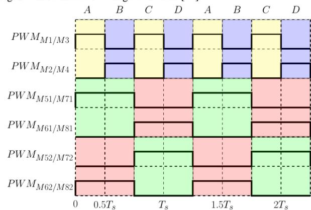
Fig. 21. Zero Inductor-Voltage Converter Gate Drive Scheme [67]
