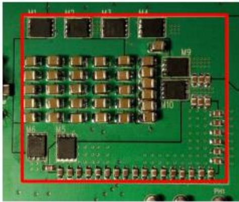
Fig. 15. 4:1 Dickson Switched Capacitor Converter Prototype, 400W/in<sup>3</sup> [35]
