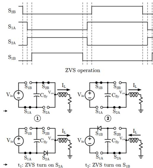
Fig. 18 Cascaded Resonant Switched Capacitor Converter Gate Drive Scheme and Switching States for ZVS Operation [2]
