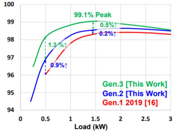
Fig. 10. LLC DCX Converter Efficiency, 99.1% Peak, 98.5% Full Load, 48V to 12V [32]
