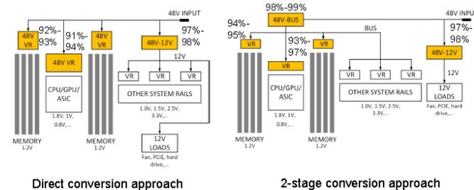
Fig. 2. A comparison of direct conversion and 2-stage conversion approach referenced from [16]
