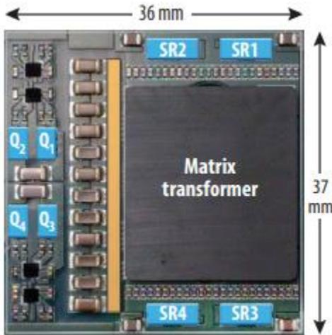
Fig. 7. EPC 900W LLC 1500W/in<sup>3</sup> Prototype [31]
