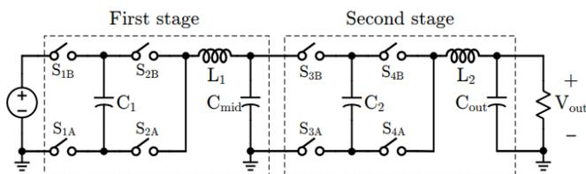
Fig. 16. Cascaded Resonant Switched Capacitor Converter [2]
