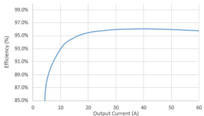
Fig. 6. EPC9130 Buck Converter - Efficiency [30]
