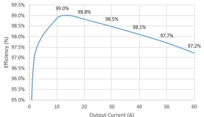
Fig. 19 Cascaded Resonant Switched Capacitor Converter Measured Efficiency, 99% peak, 97.2% Full Load 12V/60A
