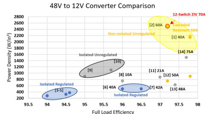
Fig. 1. A comparison of efficiency and power density achieved by various 48V to 12V DC-DC converters referenced from [15]
