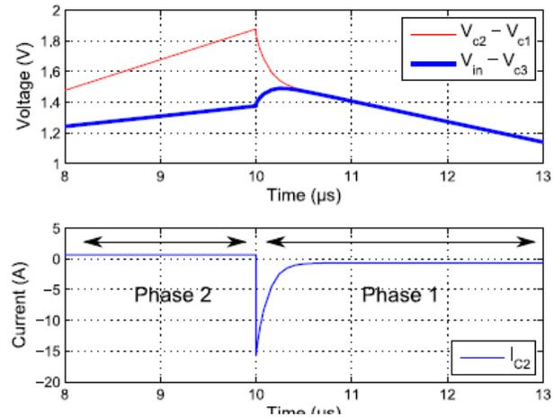
Fig. 12. Charge Redistribution in the Dickson Switched Capacitor Converter Referenced From [34]
