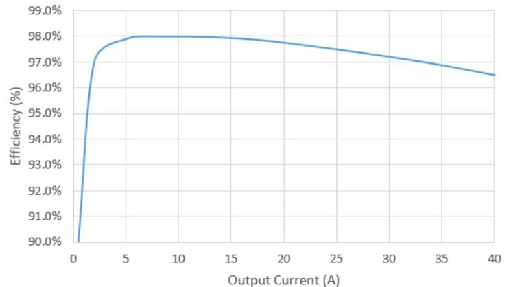
Fig. 14. 4:1 Dickson Switched Capacitor Converter Efficiency, 98% Peak, 97% Full Load [35], 48V to 12V
