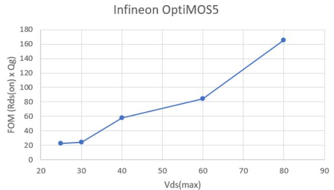
Fig. 4. Example FOM for OptiMOS5 Parts in SuperSo8 packaging
