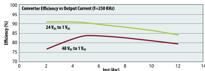
Fig. 3. 48V to 1V vs 24V to 1V Efficiency with Buck Converter [19]
