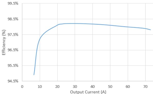
Fig. 8. EPC 900W LLC 1500W/in<sup>3</sup> Prototype Efficiency, 98.2% Peak, 97.8% Full Load 48V to 12V [31]
