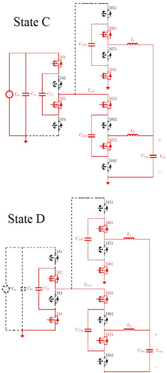
Fig. 25. Zero Inductor-Voltage Converter Switching States C and D
