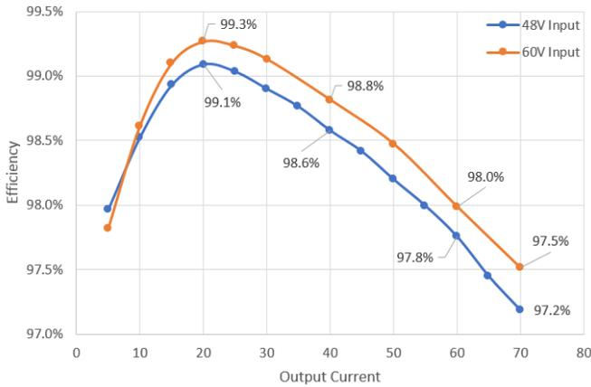
Fig. 23. Zero Inductor-Voltage Converter Efficiency, 99.1% Peak, 97.2% Full Load 12V/70A [67]
