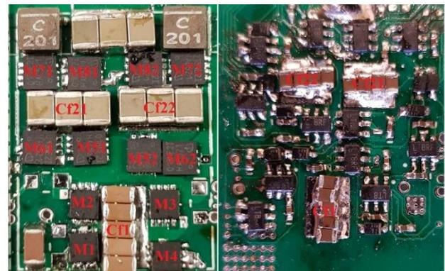
Fig. 22. ZIV Converter, One-Phase  $2500\text{W}/\text{in}^3$  Prototype [67]
