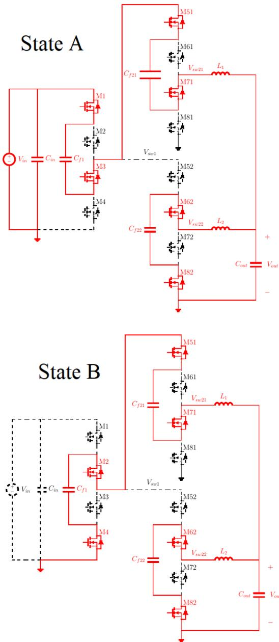
Fig. 24. Zero Inductor-Voltage Converter Switching States A and B
