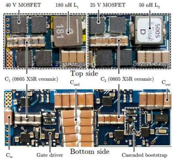
Fig. 17. Cascaded Resonant Converter, One-Phase 2500W/in<sup>3</sup> Prototype [1]
