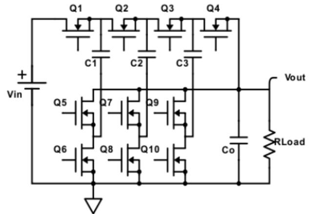
Fig. 13. 4:1 Dickson Switched Capacitor Converter [35]
