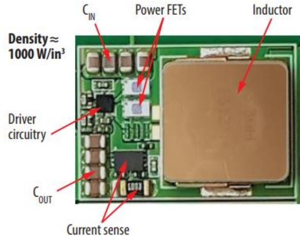
Fig. 5. EPC9130 Buck Converter - One-Phase, 1000W/in<sup>3</sup> prototype [30]
