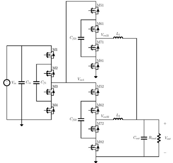
Fig. 20. Zero Inductor-Voltage Converter [67]
